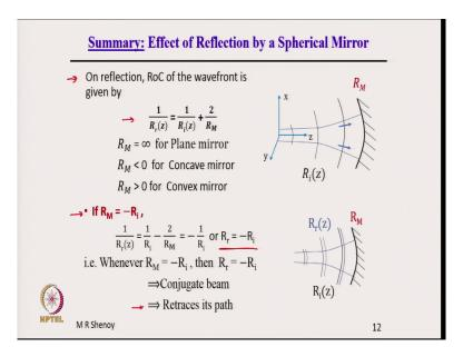
This leads us to the design problem, but before that let summarize now. The effect of reflection by a spherical mirror is on reflection. The radius of curvature of the wavefront is given by this formula, where R M is equal to infinity for plane mirror and less than 0 for concave mirror and positive for convex mirror.
