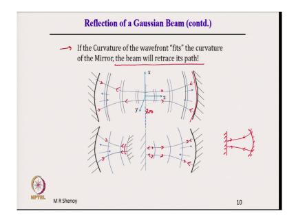
So, if the curvature, so, see the conclusion; if the curvature of the wavefront fits the curvature means magnitude is equal means what? It fits the curvature; incident beam has the same curvature as that of the mirror. So, it fits the radius of curvature, it fits the mirror here then the beam will retrace its path.
