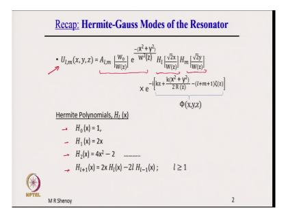
A very quick recap. So, the Hermite-Gauss modes are shown here and as I mentioned for l is equal to 0 and m is equal to 0 we have the Gaussian mode. So, this is the amplitude distribution and then the Hermite polynomials and then the phase term phi of x, y, z. The Hermite polynomials are given by this a very quick recap we have discuss this in detail.
