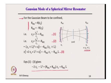
Let us see how to get this mathematically now. For the Gaussian beam from the discussion about what we have got is R M 1 must be equal to R of z 1; z 1 is the position where mirror M 1 is kept, z 2 is the position where mirror M 2 is kept. See the resonator diagram here. So, this is mirror M 1 placed at z 1 and this is mirror M 2 placed at z 2; R M 1 and R M 2 are the radius of curvature.
