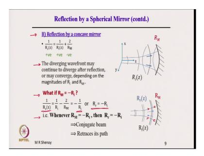
Now, let us see what happens on reflection by a concave mirror. Now, we are looking at reflection by a concave mirror this time R M is negative R M is less than 0 for a concave mirror. So, again as before we have a diverging beam which means R i is positive these black wavefronts here are positive or convex wave fronts.
