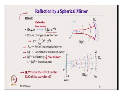
And, therefore, let us look at the reflection by a spherical mirror a very quick recall if there is a function if there is a field distribution f of x, y, z at x, y, z then the effect of reflection by a mirror is to multiply by a factor mu which can be written as mod mu into e to the power of minus i chi; chi is the phase change on reflection and mod mu is the amplitude attenuation factor.
