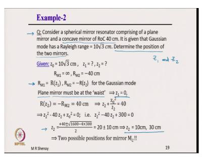
Let me take one more example, example 2. So, consider a spherical mirror resonator comprising of a plane mirror and a concave mirror; earlier I had considered one concave and one convex. So, now, I am looking at a plane mirror and a concave mirror of RoC radius of curvature 40 centimeter, plane mirror radius of curvature is infinity it is given that the Gaussian mode has a Rayleigh range of 10 square root of 3 centimeter.
