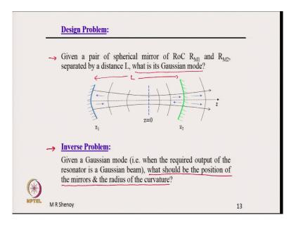
Now, let us go to the design issue. So, what is the design problem? The design problem we see given a pair of spherical mirrors of RoC radius of curvature R M 1 and R M 2 separated by a distance L, what is its Gaussian mode? How to determine the Gaussian mode? So, we have to determine the Gaussian mode for a given resonator; given resonator means a mirror of radius of curvature R M 1 is given, R M 2 is given and the separation L is given, that is a given resonator.
