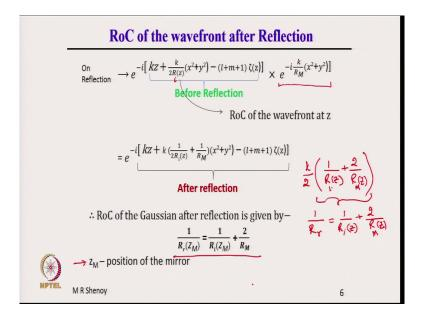
So, let us look at. Now, on reflection the incident beam, so, this is the phase term now we are looking only at the phase term because the radius of curvature of the wave front appears only in the phase term and that is why we are now looking at the phase term. So, e to the power of i kz plus k divided by twice R of z into x square plus y square minus l plus m plus 1 into zeta of z.
