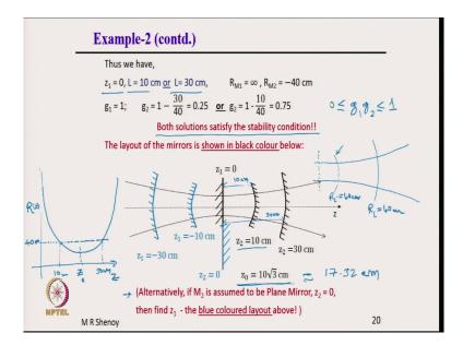
So, thus we have z 1 is equal to 0, L is equal to 10 centimeter or L is equal to 30 centimeter that is if z 2 is 10 centimeter, then L length is 10 centimeter; if the z 2 is at a 30 centimeter then length is 30 centimeter and R M 1 is infinity, R M 2 is minus 40. g 1 calculate g 1. g 1 is 1 because of plane mirror and g 2 is 1 minus 30 by 40 that is 1 plus L by R r is minus 40 therefore, 1 minus 30 by 40, 0.25 or g 2 is 1 minus 10 by 40 if you take L as 10 centimeter, then it is 0.75.
