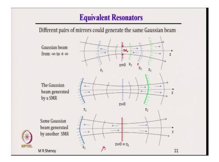
Let us continue further. Therefore, if you have a Gaussian beam one Gaussian where the wavefront is evolving like this plane then the wave front is evolving, you can place the mirrors at different positions and obtain a stable resonator. Depending on the position, the radius of curvature of the mirror should be different. In other words, if you have mirrors of different radius of curvatures and if you need a particular Gaussian, you can place the mirrors at exact positions.
