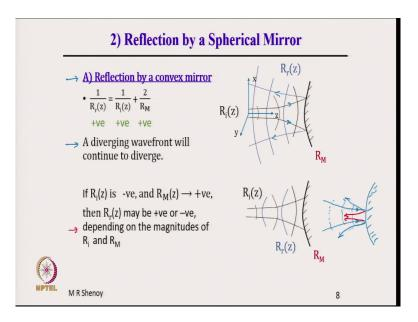
Let us take a 2nd example, reflection by spherical mirror. Here there are reflection by convex mirror and concave mirror. So, first consider reflection by a convex mirror.
