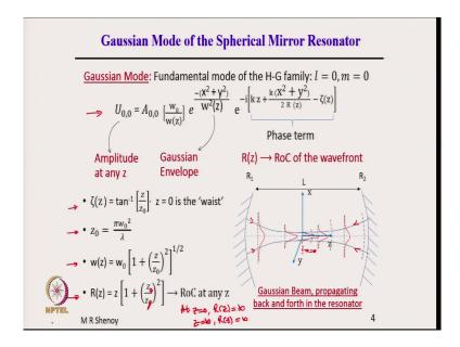
So, the Gaussian mode of the spherical mirror resonator it is the fundamental mode of the Hermite-Gauss family. So, we have already repeated this. The amplitude at any z, the Gaussian envelope term here and where zeta of z is equal to tan inverse of z by z naught, z is equal to 0 is the waist. So, we can see here in the resonator, the Gaussian beam is going back and forth is going back and forth.
