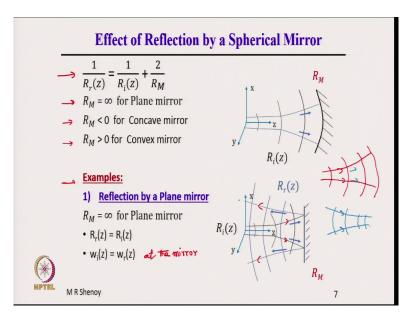
So, the effect of reflection by a spherical mirror is here now, the same formula. 1 by R r of z is equal to 1 by R i of z plus 2 by R M of z. Note that R M is equal to infinity for a plane mirror and therefore, in the case of a plane mirror we can immediately see that if R M is infinity then R r of z will be equal to R i of z that is the first example which is shown here reflection by a plane mirror.
