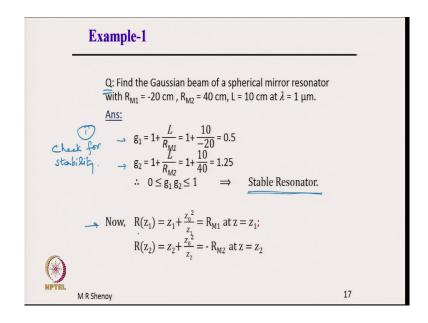
Let us take some examples and it will become very clear now. Question: find the Gaussian beam of a spherical mirror resonator with the R M 1 is equal to minus 20 centimeter which means this is concave mirror; R M 2 is 40 centimeter which means this is convex mirror and L is equal to 10 centimeter at lambda equal to 1 micrometer.
