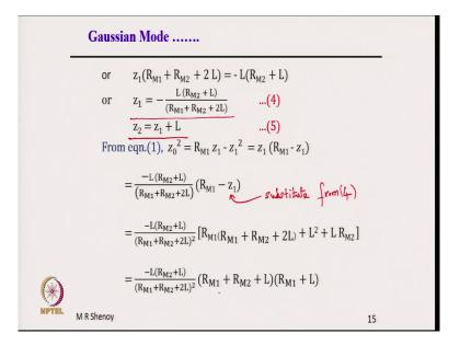
Now, let us simple algebra here that is  $z \ 1$  into we have taken  $z \ 1$  terms together is equal to L into this or  $z \ 1$  is equal to a formula which is obtained here by simple starting point is simply this. This is the starting point which we have conceptually discussed and then you simply substitute for this and simplify this simple algebra to get  $z \ 1$  is equal to that and  $z \ 2$  is given by this.
