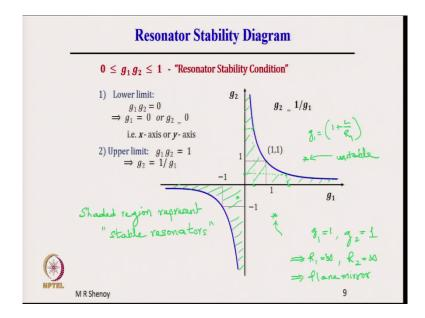
So, that is what is shown in this slide. So, the lower limit g 1 g 2 equal to 0. So, g 1 is equal to 0 or g 2 is equal to 0; the resonator stability diagram is a diagram, where one of the g, that is
