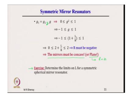
So, for the symmetric mirror resonators, g 1 is equal to g 2 and therefore, equal to let us say equal to g equal to g. Therefore, we write 0 less than or equal to g square less than or equal to 1; which implies g will lie between minus 1 and plus 1 that is minus one less than or equal to 1 plus L by R less than or equal to 1 or this implies 0 less than or equal to. So, we have added plus 1 to all the sides; 0 less than or equal to 2 plus L by R less than or equal to 2.
