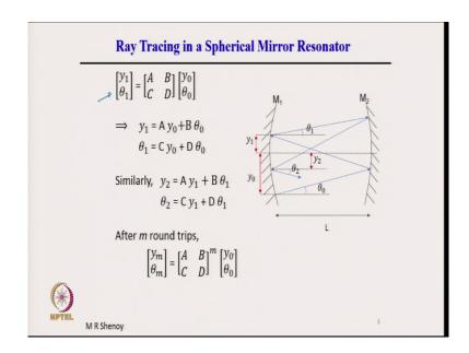
Now, let us look at ray tracing in a spherical mirror resonator. So, as discussed, the ray coordinates y 1 and theta 1 after one round trip is given by the matrix equation here; that means y 1 is equal to A into y 0. So, row into column plus B into theta 0. And similarly theta
