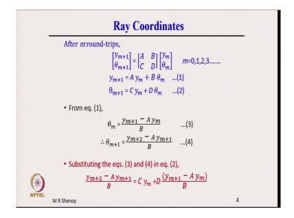
And therefore, after m round trips, the coordinate y m plus 1; the new upgraded coordinates, y m plus 1 theta m plus 1 is still related to y m and theta m through the A B C D matrix.
