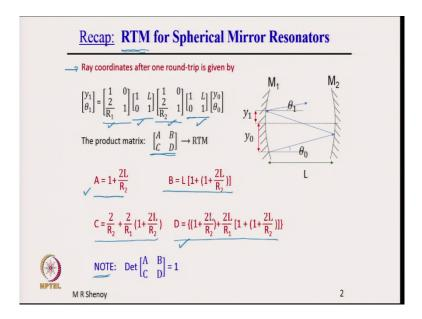
Now, let us quickly recap, a quick recap of what we had done. So, we obtain the ray transfer matrix RTM, here ray transfer matrix for a spherical mirror resonator. What we have done is, the ray coordinate after one complete round trip involving four operations. So, we start with y 0 theta 0. So, y 0 is the displacement from the axis here and theta 0 is the angle that it makes with the horizontal, in this case the optic axis of the system.
