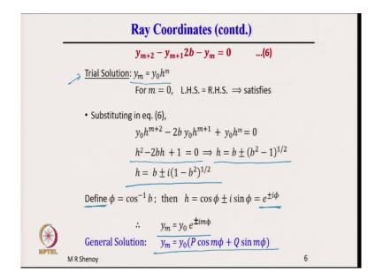
So, let us look for trial solution of this equation; we want to look for solutions of this equation. So, we start with a trial solution. So, a trial solution can be written as y m is equal to y 0 into h to the power m. Note that this satisfies for m is equal to 0; for m is equal to 0, it is y 0 equal to y 0, that is LHS is equal to RHS and that satisfies.
