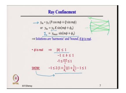
Now, let us go further and discuss. So, y m therefore, is equal to y 0 into P cos m phi plus Q sin m phi, which can also be written in the form; we can combine these and write in the form of y 0 into some constant K sin m phi plus phi 0. And y 0 into K if we designate this as y max; then we have y m is equal to. So, we have y m is equal to y max into sin m phi plus phi naught.
