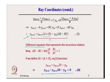
So, let us simplify that further. So, that gives y m plus 2. So, this is the equation, you simplify this; this comes out to be y m plus 2 minus A y m plus 1 is equal to as written here. And therefore, y m plus 2 is equal to y m plus 1 into A plus d.
