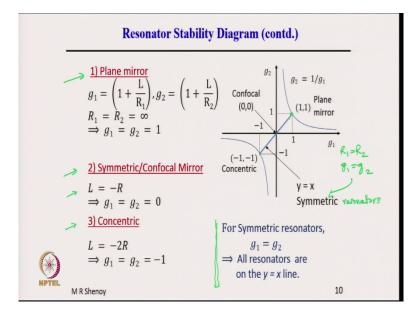
Let us look at other resonators, some more examples. So, here it is, the plain mirror resonator has g 1 is equal to g 2 is equal to 1 and therefore, we have this equal to 1. So, this is the point which corresponds to a plane mirror resonator. Now, for all symmetric resonators g 1 is equal
