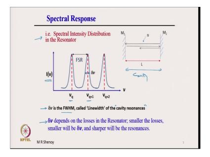
Now, the spectral response refers to the spectral intensity distribution in the resonator. That is spectral intensity distribution means, intensity distribution as a function of frequency of the radiation inside the resonator that is if we plot the intensity inside the resonator as a function of frequency then; obviously, at the resonance frequencies we will get maximum intensity.
