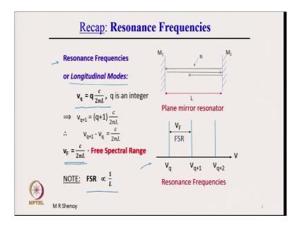
A very quick recap. So, the resonance frequencies or they are also called longitudinal modes of a laser are given by nu q is equal to q into c by 2 n L where q is an integer. We have seen that in the case of laser resonators q is generally very large number 10 to the power of 5 10 to the power of 6 and so, on.
