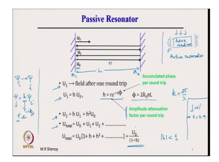
Now, let us consider a passive resonator right now we are looking at the optical resonator which is a passive resonator. So, passive means there are no active medium inside the resonator. So, if you have a resonator with an active medium inside, then this is called an active resonator particularly when the active medium is pumped.
