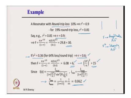
Let us take an example consider a resonator with a round trip loss of 10 percent. Round trip loss of 10 percent what does this mean? This means round trip loss refers to loss of energy in all optical measurements we measure energy or power or intensity.
