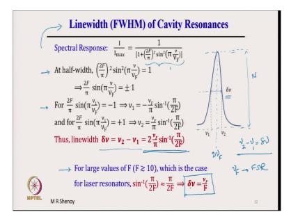
Finally, we come to the line width of the cavity resonances. Line width refers to the full width at half maximum of these resonances. So, it is illustrated here. So, this is the resonance and the frequency resonance frequency is q times nu F is the resonance frequency.
