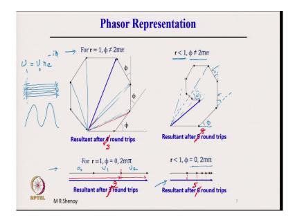
So, let us look at a situation where r is equal to 1 which means there is no amplitude attenuation factor. So, recall that U 1 is equal to U 0 into r into e to the power of minus i phi that is h. If r is equal to 1, the magnitude of U 1 is the same as magnitude of U 0 which means all these magnitudes are the same, but phi the round trip phase phi is not zero or integral multiple of 2 pi when phi is finite then if we start adding them we can see the phasor after two round trips.
