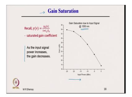
So, the gain saturation what is shown here is the input signal power at a particular wavelength. This is at the wavelength 1550 nanometer what is shown in the previous slide is at different wavelengths, the gain is measured for different input powers. Input power is varied at a given wavelength the power is changed and the gain is measured for different input powers and this is plotted for different wavelengths this is carried out for different wavelengths.
