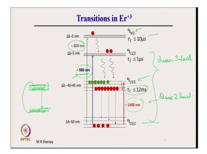
And therefore, the transitions will be like this the energy difference from the ground state 4 I 15 by 2 is the ground state to this level corresponds to a wavelength of about 800 nanometer this is the largest difference. And, this the difference here corresponds to 980 nanometer from ground state to the third level and the difference from here to the second level corresponds to 1480 nanometer. These three wavelengths can be used to excite atoms from the ground state to the upper state.
