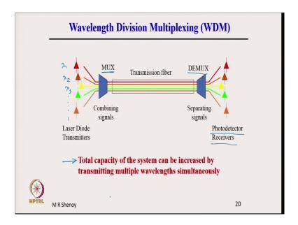
Finally, a very important application of the erbium doped fiber amplifier is in wavelength division multiplexed systems for optical fiber communication. An application which I would probably discuss towards the end of the course, but the point I wanted to show is the following.
