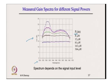
So, this is actually a measured spectrum in our laboratory. So, what is measured is wavelength verses gain as you can see different levels of input power. This is P s is the signal input power 8 microwatt 32 micro, as the signal power increases you note that the gain profile decreases.
