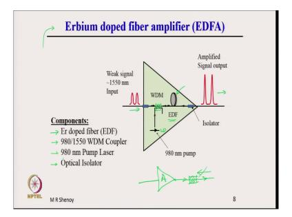
Now, I come to the erbium doped fiber amplifier a little bit about the amplifier system itself. So, the amplifier here is a schematic of the erbium doped fiber amplifier. So, what is shown is input signal weak input signal around 1550 nanometer. Why around 1550 nanometer?
