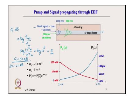
Now, it is again illustrated here with some more numbers as you can see the 1550 field here shown with small amplitude because it is a weak signal. Because the purpose of the amplifier is to amplify input weak signals to get sufficiently strong signals at the output. And, if we
