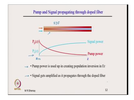
Now, the evolution of the pump and signal are schematically shown here. So, this is the optical fiber. Both pump and signal are input at this end, this is the doped fiber EDF. So, this is the EDF erbium doped fiber. The pump as you see the red color continuously reduces because the pump got absorbed in creating the population inversion.
