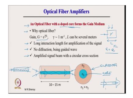
First optical fiber amplifiers; an optical fiber these comprise of an optical fiber with a doped core, core is the central region of a fiber core forms the gain medium. The doped core in an
