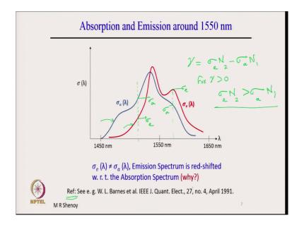
So, this is what is illustrated the actual absorption and emission cross-sections of the erbium ions in silica around 1550 nanometer. So, what is shown is the absorption spectrum. So, this is the emission cross-section of for absorption. So, the cross-section is of course, represents the strength of absorption at a given wavelength.
