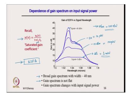
Here what is shown is the dependence of gain spectrum on the input signal power. So, what is shown first let me indicate what is shown. So, these are different curves for different signal powers so, different values of signal powers. So, this is the first one is shown here for minus 40 dBm minus 40 dBm is 1 microwatt.
