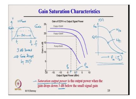
The gain saturation characteristics of an amplifier typically the gain saturation characteristics are shown here for three different values of pump power. As I mentioned if you change the pump power even at the beginning when we discussed about the gain coefficient you may remember that we had a saturation saturated gain varying like this.
