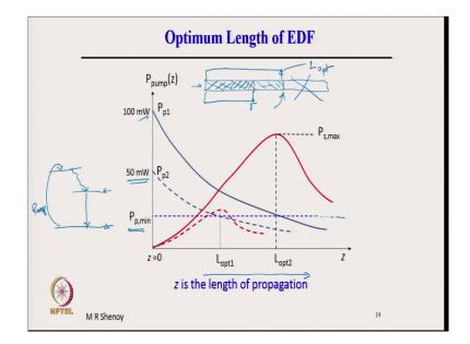
There is one important concept in this amplifier is the optimum length of EDF what is this. So, what is shown is the in this direction we have the length of propagation. Let us consider the input power as 50 milli watt at the input at Z is equal to 0. As I already explained the pump exponentially drops down because it continuously increases it continuously is absorbed and the signal from a small value here continuously gets exponentially building up.
