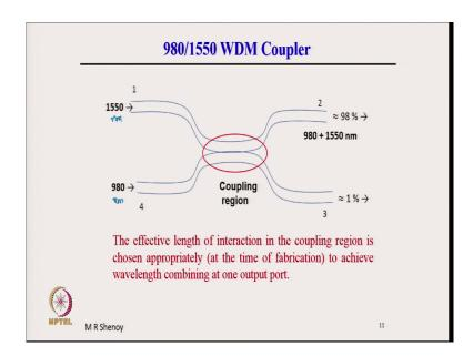
So, you can see the diagram more carefully if you put 980 from here this an optical fiber component a very compact component. So, if we put 1550 nanometer wavelength here that is the signal and the pump wavelength 980 nanometer here, then they will combine at one of the
