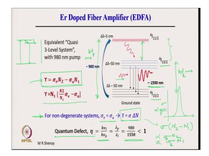
So, erbium doped fiber amplifier as I have discussed in the previous slide equivalent quasi 3 level system with 980 nanometer pump, atoms are excited to 4 I 11 by 2 from there they rapidly come down to 4 I 13 by 2 and a signal population inversion is created between 4 I 13 by 2 and 4 I 15 by 2.
