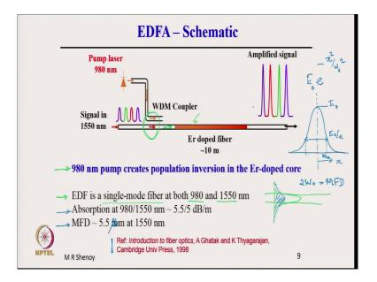
So, the schematic is represented here. So, you have a pump laser and this is again the coupler is here the WDM coupler which. So, the weak signal and the pump both are combined into one fiber which enters the erbium doped fiber. This red portion here is the erbium doped fiber may be typically 10 meters in length.
