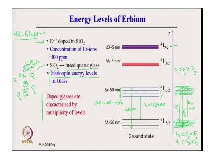
The energy levels of erbium. So, let us very quickly recall I had discussed in detail the energy levels, the nomenclatures in the case of neodymium doped YAG. And here I have directly written the erbium doped silica fibers or EDF where erbium appears as a Er plus 3 ions and these are the energy levels of the Er plus 3. So, as before you can see 4 which is 2 s plus 1 multiplicity of the levels and I is the orbital angular momentum and 9 by 2 in this here represents the j value.
