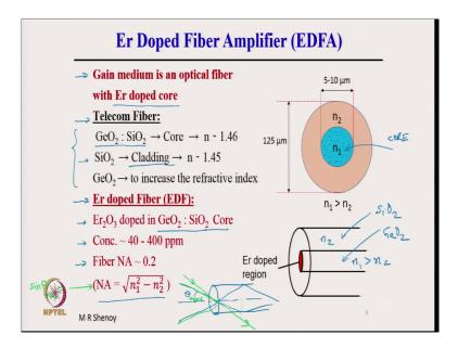
Now, let us come to erbium doped fiber amplifier that is about general fiber amplifiers. Erbium doped fiber amplifiers where the gain medium is an optical fiber with the erbium doped core. So, erbium is a rare earth element, normally in telecom fibers. So, erbium doped core means again we have shown here the cross-section whereas, where this is the core and therefore, this core is doped with erbium.
