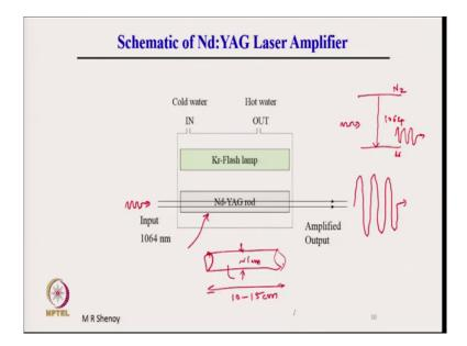
Let us continue a typical schematic what is shown is a schematic of Nd YAG laser amplifier, how does it look like? So, typically there is an Nd YAG laser rod this is a rod which is generally about 1 centimeter in diameter and 10 to 15 centimeter in length in a practical system. So, this L is generally 10 to 15 centimeter and the diameter is approximately 1 centimeter of the order of 1 centimeter.
