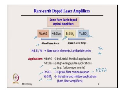
Rare earth doped laser amplifiers; some of the rare earth doped optical amplifiers which are widely used are Nd YAG laser amplifier, Nd glass neodymium doped glass and erbium in silica and ytterbium in silica. These two the second erbium silica and ytterbium in silica are widely used as fiber amplifiers.
