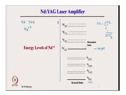
So, let us first start with the Nd YAG laser amplifier. So, what is shown here is Nd levels of energy levels of neodymium because in Nd YAG when we say it is Nd doped in YAG YAG is Yttrium Aluminium Garnet. So, it in YAG it is replacing the ytterbium here yeah yttrium here, why? It is replacing the yttrium and therefore, it exists as Nd plus 3 ions and what are shown here are the energy levels of the Nd plus 3 ion.
