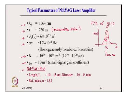
Finally typical parameters of an Nd YAG laser amplifier. So, the wavelength of operation is 1064, depending on. The host it may slightly vary the upper level lifetime is given here 230 nano second, so this is the lifetime of the metastable state. So, this is the metastable state sigma e is the emission cross section typical numbers I had mentioned that it is of the order of 10 power minus 23 minus 24 meter square.
