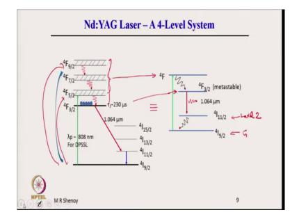
So, if we look at the equivalent picture now let me simplify this. All of this here the same diagram I have shown all of this. So, you are pumping from here to any of the levels; any of the levels all the atoms would trickle down and come and accumulate here. Therefore, the role of these levels is simply to populate this lowest level and therefore, this level is our 4th level, in a four level laser that 4th level is these multiplex of levels are equivalent to the higher level.
