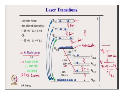
So, let us continue from here. So, let us now come to the laser transitions of an Nd YAG laser. How does the Nd YAG laser amplifier work the scheme of amplification? So, we have
