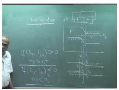
And the band diagram now so originally it was like this, so now it has been lifted up from the original position relative to that, so this was it is original position, so let me not show the original position, so this is after forward biasing so forward biased junction what happens to the Fermi function, so Fermi level in this side remains where it is far away from the junction there is no potential felt, so Fermi level is here.
