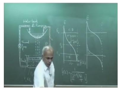
So, we have at thermal equilibrium again let me plot Ev, Ec and E versus f (E) the Fermi function and you have a distribution, so this is 1.0, so it is 0.5 f (E) equal to 0, 0.5 you draw the vertical line where it intersects that gives you Ef. So, this is at a particular temperature t, t greater than 0 1 f(E) describing the probability of occupation of the conduction band and the valance band and f(E) is given by 1/E to the power E-f/kT+1.
