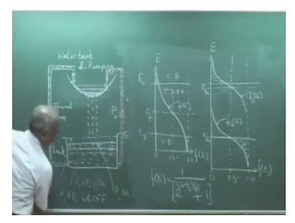
I could have kept a drawn figure already for display but I thought if I plot it in front of you you will know what is the difference. So, this is Efc Fermi level or Fermi function describing the conduction band occupation probability of the conduction band this part has no role only this upper part has a role to describe the population of the conduction band occupation probability of electrons in the conduction band.
