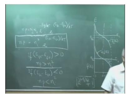
And therefore N into p is equal to Nc into Nv into the product of these is equal to E to the power –Eg/kT N into p is Nc into Nv E to the power Ev E to the power –Ec therefore it is –Ec-Ev therefore –Eg/kT into what do we have there is a second term E to the power let me go further into E to the power Efc-Efv/kT what is this term it is Ni square this term is Ni square therefore this is equal to Ni square into E to the power Efc-Efv/kT, so N into P is equal to this/kT.
