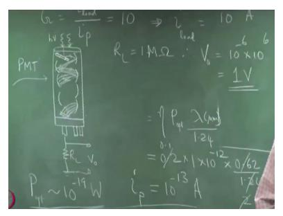
So gain which is = i at the load resistance, output current/i primary. This is = 10 to the power of, the number which we have calculated here, and therefore the current generated this implies i load=iP is 10 to the power of -13, so this is simply 10 power -6 amperes, i load=10 power -6 amperes. So recall that we have a tube. The PMT normally looks like this. There is a tube and a window at the top for photons to incident. So this is incident photons. It is the tube.
