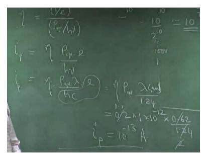
So I go by the definition of quantum efficiency=electron flux, so i/e/incident photon flux P optical/h nu, incident photon flux and therefore this is the primary photo current generated with this eta here. Therefore, we have i, the primary photo current=we have eta\*P op/h nu\*e, so that is = eta\*P op/h\*C/lambda\*e and we know this quantity here hC/e is 1.24 if lambda is in micrometer. So this is = eta\*P op\*lambda in micrometers now/1.24.
