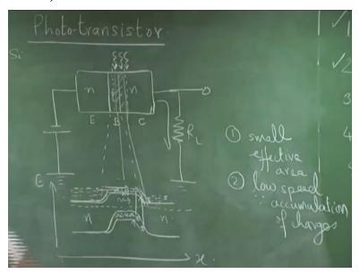
Photo transistor basically is a transistor. We consider an NPN transistor here. That is a silicon NPN transistor. The incident light is incident at this junction. The light incident at other junctions do not really contribute to the current and therefore the active junction is this one. So this is an NPN transistor. This is the emitter, this is the base and collector. So usually this end is forward biased and in a photo transistor normally, this is the load resistance.
