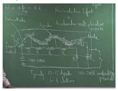
Photomultiplier, the basic principle of operation is first photoelectric effect, photo-emissive type of detector. Photoelectric effect which is followed by Avalanche multiplication process. The photoelectric effect + Avalanche multiplication process, so let me illustrate the simple basic schematic of a PMT and then we will discuss in detail. This is a photo cathode. Photon is incident through a filter or a window.
