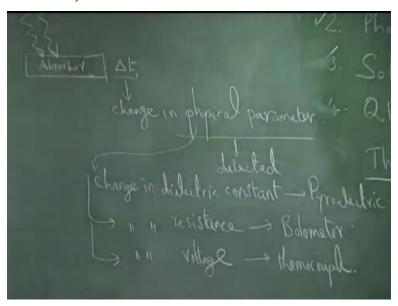
The basic idea is simple that there is an absorber, appropriate absorber. The incident radiation leads to a change in temperature delta T. This is the absorber. So delta T leads to a change in physical parameter of this material absorber here and this change in physical parameter is detected. So what is the change in physical parameter, what all parameters could be changing. For example, this physical parameter could be a change in dielectric constant.
