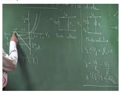
Basically, this is PN diode or PIN diode and if we recall, the IV characteristics of the photo diode, then we have, when there is a photon flux, which is incident, then we have the scales on
