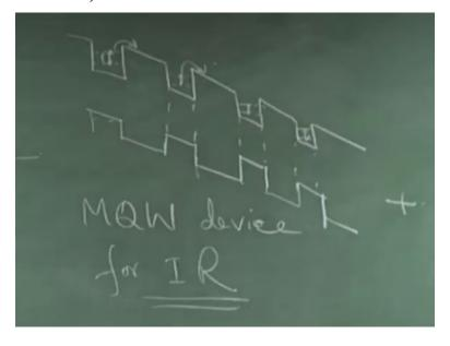
Similarly, on this side, so here are the wells. In each of the wells, we have the same energy difference provided they are identical. If the well width is the same everywhere, if they are identical, then the energy separation here between the 2 sub-band levels is the same everywhere and therefore the photon of same energy can be absorbed. So the electron makes an upward transition and then a transition outward.
