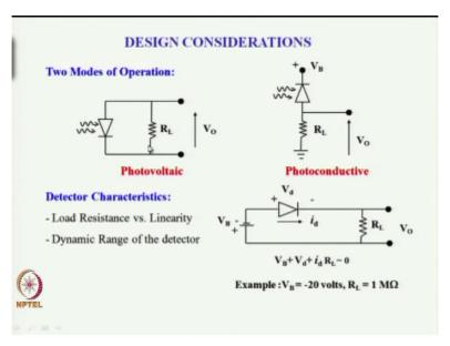
In particular, we discussed that there are 2 modes of operation photovoltaic and photoconductive mode of operation and we have discussed in detail the design characteristics here and how to choose the load resistance.
