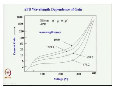
This is characteristics which shows the wavelength dependence of current gain the typical silicon APD current gain here. And you see that at lower wave length here the current gain is smaller and as the wave length increases up to around 1 micron or 1000 nanometer the current gain increases. This increase is this low value of current gain and higher values of current gain here are primarily because of the quantum efficiency.
