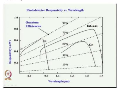
So silicon it has a smaller quantum efficiency at lower wave length and the quantum efficiency is relatively large the responsivity is large as the wave length increases. Of course once as we reach near the band gap wave length the quantum efficiency drops down and this
