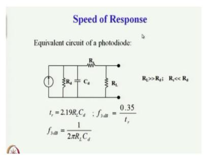
So a small topic of importance is also speed of response of PIN photo diodes here and the equivalent circuit of a typical diodes here is shown in this diagram here. This is a current source with resistance across the diodes resistance the reverse diode resistance which is a very large resistance. And a Junction capacitance here the diode capacitance which is the CD or CJ and a series resistance and the load resistance.
