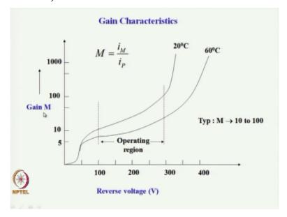
The gain characteristics of a typical APD is shown here reverse voltage the numbers are here now. Typically, 100, 200, 300 volts are applied for as the reverse-biased and what is plotted is the gain the current gain M. M is defined here iM./iP. This is the gain after the multiplication process and this is the primary photo current due to the incident photon. So at 20 degree centigrade for example 20 degree Celsius the current gain increases initially as the voltage increases.
