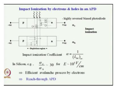
So let me discuss in the next slide here and then come back. We can see that there is a parameter called impact ionization coefficient alpha which is defined as 1/L internal average. This here refers to a collision the distance the average distance travelled between 2 successive collisions so this is L impact. So the average distance 1/L impact is called the impact ionization coefficient this is per unit length.
