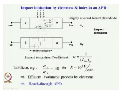
In fact, if we look at the previous diagram here please see that a carrier pair generated here electron gets accelerated in this direction, hole get accelerated in this direction. As the electrons proceed it creates additional electron hole pair and the hole which proceeding in this direction creates additional electron hole pairs. So an electron which is created here electron hole pair electron moving in this direction will keep on creating additional electron hole pairs.
