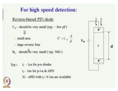
And therefore for high speed detection reverse biasing much helps reverse-biased PIN diodes are used for high speed photo detectors CD here should be very small because it is in the denominator if you want to have a large cut off frequency typically few (()) (08:34) and Cd will be small. If you have a small area and large reverse-biased leads to a small junction capacitance because the depletion region width of the depletion region increases small area of the photo detector here.
