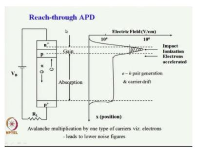
We will see what is this Reach through APD. Here is the APD structure a high n + region then a P region here and pi that is (()) (22:41) near intrinsic or (()) (22:43) here p and then this is the p p+. So because of a large n + so there is a reverse-biased here applied because of high doping concentration here at this junction close to the junction we have large density of immobile positive ions because the electrons have migrated here.
