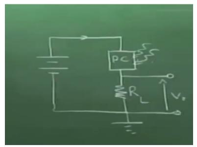
So, you have a supply here and here is the photoconductor, the different designs, so this is the photoconductor and is a load resistance, so the whole thing is grounded and here is the output, so vo. The output taken across a load resistance and this is the photoconductor, so incident; light is incident on the photoconductor; light is incident on the photoconductor with changes the conductivity of this element.
