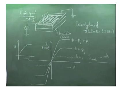
So, how do you think the IV characteristic would look like? It is a simple piece of semiconductor and you have applied a current, so the IV characteristic of the photoconductor looks like this. So, this is what I have shown by dashed line is when; okay let me draw completely, so what I am plotting is the I, the photocurrent IP verse the applied voltage v. So, you have; so this is with phi = 0, phi = phi 1 and phi = phi 2, which is > phi 1.
