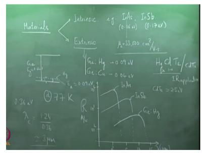
Now, let us come to materials, which are use so long, I did not discuss about materials, so materials; generally, photoconductors are used to; generally, these are used to detect long wavelength materials and therefore there are 2 types or 2 kinds of materials which are used, they are, intrinsic and extrinsic. As you know intrinsic normally refer to pure semiconductors and extrinsic refers to doped semiconductors.
