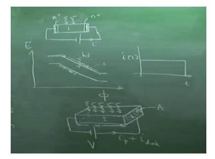
Typically it is a; the photoconductor is typically like this, they normally use a metal contact here let us say metal and therefore for ohmic contact, you normally use n+ here and then an intrinsic medium and n+, it is only for contacts sake, this is metal, so this n+ and intrinsic, so the carriers are photon flux is incident here, there are better designs but I am just explaining that there is; so, if you draw the band diagram of this, so you n+, which means the electron thermi level is here.
