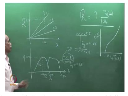
And if we plot the responsivity therefore so responsivity versus lambda if you plot R here then you would have straight lines or different values of eta. So, this is what we have plotted eta=1 may be 0.6, 0.3, and this is with wavelength. So, you can see the typical numbers when lambda=1.24. So, if take lambda here as 1.24 and eta=1 then responsivity here must be 1. So, lambda=1.24 then responsivity will be = 1.
