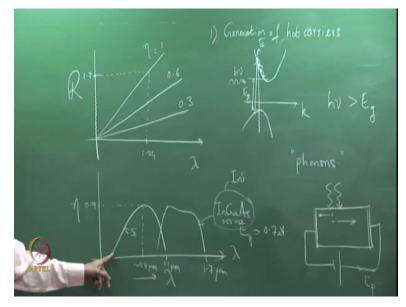
So, first because of generation of hot carriers if you take the band gap here so this is ek (()) (10:11) so k versus E. I have drawn an indirect band semiconductor to indicate that it is silicon for example. And when the energy is larger for example this is the Eg, for h nu incident photon energy much greater then Eg electron transition can take place an electron can make an upward transition to an allowed state here.
