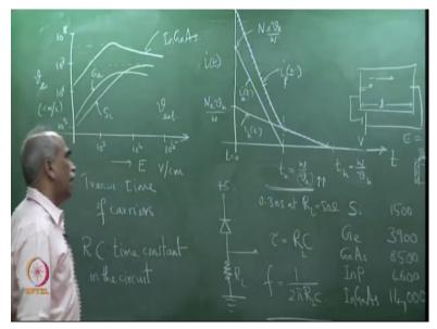
Electrons moves, holes move when you apply a field before you apply a field it just does not move there is nothing. So, that is why we have applied a field. So, you have applied a field here. So, if you applied a voltage V and this is d then you have E electric field, E=v/d. So, there is a electric field which is applied as you increase the voltage the electric field is increasing. The electron is getting drifted rapidly.
