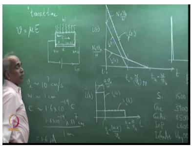
Now the photons are incident everywhere not at one point over the entire detector surface what will happen at every point electron whole pairs are generated. And electrons which is generated here is instantaneously collected. Where are electrons which is generated here will take a time t=w/v is the total time and so if I plot ie of t, please see this. So, this is time versus i\*t. So, first let me plot ie\*t. So, it will be largest at t=0 because all the electrons are moving.
