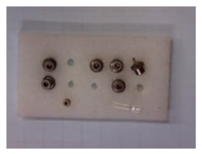
An LED which is 2-pin diode, light emitting diode and this is a spoilt one, so I can touch that, but it is important that you see that there are 3 terminals there. There are 3 terminals and these are the same 3 terminals here, 1, 2, 3 and that is the bottom view and the top view as you can see, there is a glass window in each one of the devices. This is the laser diode used in CD writing device.
