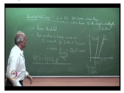
So quantum well lasers, lower thresholds, less sensitive to temperature variations, lower threshold currents. This can be quantified by, if you recall, that the character I had introduced a characteristic temperature T0 which is approximately 140 K for gallium arsenide Fabry-Perot lasers, FP lasers. We have discussed this earlier. This is the order of 400 K for same gallium arsenide quantum well lasers.
