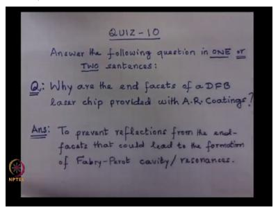
The answer is, here is the answer. To prevent reflections from the end facets that could lead to the formation of Fabry-Perot cavity or resonances. It is very clear that AR coating as the name indicates, it is an antireflection coating to block reflections coming from the ends. If the reflections come from the end, there will be feedback from the ends and the cavity will also form a Fabry-Perot cavity and therefore there will be allowed resonances at those frequencies.
