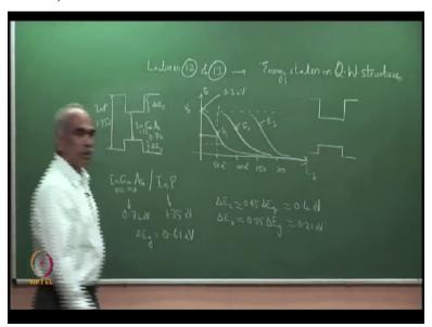
So this point I would like to illustrate with the help of an example, a very important laser material combination used is indium gallium arsenide versus indium phosphide substrate. So this is high n 0.53, gallium 0.47 and arsenic. Why we chose this combination is? This material is lattice matched to indium phosphide. So it is a lattice matched combination. The band gap Eg of this is approximately 0.74 eV.
