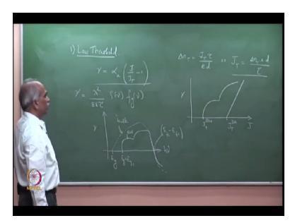
Low threshold, the first point. Let me now discuss the first point. Why do we have low threshold? If you recall, we had an expression for delta nT=JT\*tau/e\*d or JT=transparency current density=delta nT\*e\*d/tau, d is the thickness of the quantum well structure and then if you plot the gain coefficient, JT and if you see the gain coefficient gamma=alpha a\*J/JT-1. In the case of quantum well structures, JT, d is very small compared to double heterostructure structure.
