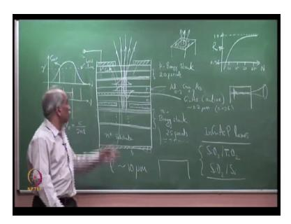
Recall that the gain spectrum of the semiconductor is this and the cavity resonances are here. These are the cavity resonances with a free spectral range here. So in both the cases, the axis is new. So this axis is frequency nu, this is gain gamma, and this is resonance frequencies nu and this is the free spectral range nu F=C/2n\*1. Unlike the case of bulk semiconductor lasers, here 1 is very small, 1 is of the order of 10 micrometer which means nu F, the free spectral range is large.
