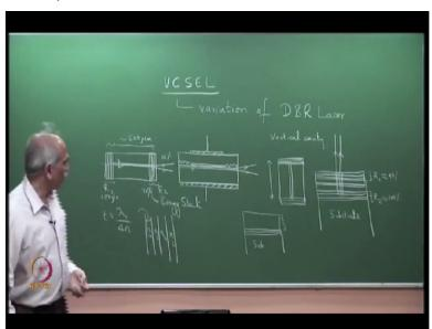
We can think of this as a variation of DVR laser. In the last class, we discussed about DFB and DBR laser, distributed Bragg reflector laser. So recall the DBR structure, there is the active region and there are corrugations here that is periodic structure. The frequency is selective, periodic corrugations there and this is the DBR and I had discussed that this was basically to have a cavity here, a Fabry-Perot.
