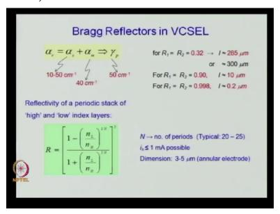
1-n low/n high to the power 2n/1+n low/n high to the power 2n whole square. So that is the reflectivity of a Bragg stack, a periodic structure where N is the period, capital N is the period. So if I plot N here versus reflectivity, typically the reflectivity varies like this. This is 1, 1.0 and here, this is approximately 0.96. This is 10 20 25 15. So what I have plotted, please see is, see this graph clearly.
