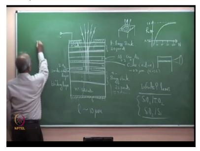
Now why did I write this? So one is approximately 500 angstrom and another is 560 angstrom. So if you add lambda, the period, please see the period here, this is lambda period is = t1+t2 with is = t1+t2=560+500=1060 angstrom. So 1060 angstroms is 106 nanometer or equal to nearly equal 0.1 micrometer, is the period. So typically people use here 25 periods and for the upper Bragg stack here, I also have an upper Bragg stack which is there in the diagram, okay.
