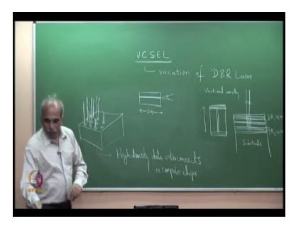
Because then on a chip like this, on a chip, you can grow large number of lasers all emitting to the top, upward. So this is the top view I am showing. So all of these giving light like this. It is an array of vertically emitting from the surface, lasers emitting from the surface. You can make an array of lasers. There are several applications of such arrays including pumping to other lasers.
