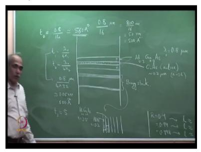
So let me draw it here. You have, because there is one more layer in between which is mixing. So I will show that. So you have the active layer here which we normally show by dotted line. Outside this is the cladding region. So this is the one which forms the double heterostructure. A low band gap materials sandwiched between higher band gap material, all right. In simple terms, this could for example, this is a gallium-arsenide laser, then this is gallium arsenide active layer.
