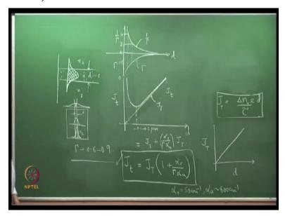
Now let me plot this gamma, how this gamma look like with d. So first thing is here, this is the expression, J and T is here, let me erase the rest of them. I want to plot and see the importance of this confinement factor in determining the threshold current. What I am now plotting is d versus gamma. So gamma, minimum value is 0, maximum value is 1. So for very small values of d like this, the mode is spreading, gamma is closer to 0.
