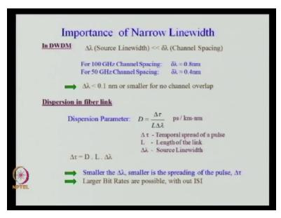
So to be familiar with the numbers, so there is a slide particularly this is importance of narrow linewidth in optical communication. There are importance of narrow linewidth in various applications, a smaller narrow linewidth gives you a higher coherence and a highly coherence sources are required for various applications but the importance which is discussed here is with the respect to optical communication.
