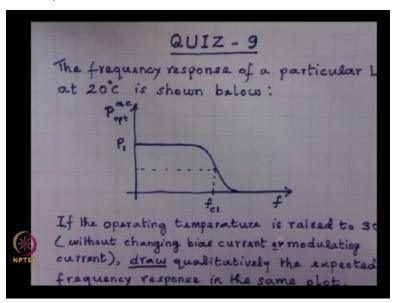
So this was the quiz question. The frequency response of a particular LED at 20 degrees is shown below. If the operating temperature is raised to 30 degree without changing bias current or modulating current or without any change, draw qualitatively the expected frequency response in the same plot. So what you see is when the temperature goes up from 20 to 30, 2 things happen.
