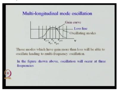
So little bit more about towards, we are going towards selection of a single frequency. So this we have discussed, there is a gain curve here. The vertical lines are allowed resonance frequencies of the resonator. So those modes which have gain more than loss, will be able to oscillate leading to multi-frequency oscillation of the laser. So in this figure, oscillation will occur at 3 frequencies because you can see 1, 2, 3. For these 3 frequencies, gain is more than the loss.
