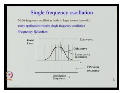
Single frequency oscillation. Therefore, if you somehow modulate the loss, here is the concept. If you somehow make loss very high for all frequencies but the required frequency, then that frequency alone will oscillate. So what is shown here is gain curve is the same but the loss line is now up except for 1 frequency where the loss has dropped. Why it has dropped, we will see but if I make, this is just the principle, principle of selecting a single longitudinal mode.
