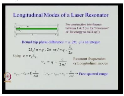
The longitudinal modes of a laser resonator, we have discussed this and therefore I quickly go through it. We already discussed this on the board for constructive interference between 1 and 2, which means after 1 round trip, that is for resonance or energy build-up, round-trip face must be integral multiple of 2 pi, we have discussed this in detail in lecture 33, 2 is an integer and therefore you get an expression for the resonance frequency nu q which is equal to q into this.
