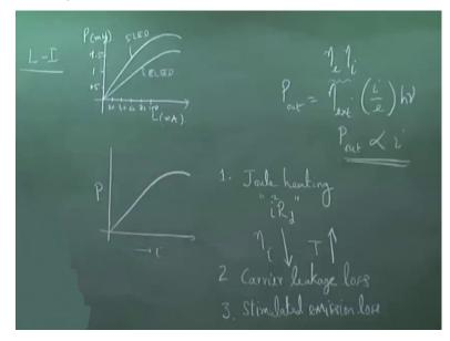
So L-I characteristics, L-I or i-P okay, so what do we expect so current I through the diode versus optical power, so P optical. What do we expect? We expect a linear curve because we have already derive the expression that P out=eta external quantum efficiency\*i/e\*h nu, therefore, P is proportional to P out is proportional to i. So we expect a linear characteristic here, so do we get linear characteristics many of you have measured this, this is not wrong.
