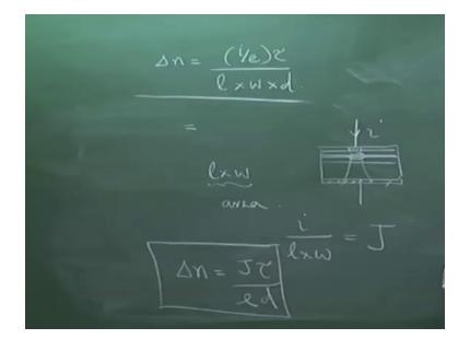
So this if you recall 1\*w, what is 1\*w? Length\*width gives you the area of the strip, 1\*w gives you recall the active region, so before erasing I should have checked. So this is now front view okay cross-section, so here is the strip metallic strip and under this so many layers are there alright, let me know the layers again very quickly okay, so the carriers are flowing like this and this is the active region here, this width is w and l is the length.
