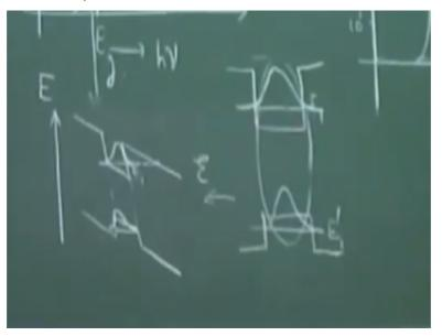
So if you recall the quantum well structure here a single quantum well showing you a single quantum well and there is the wave function here correspond this is the lowest state and you have a wave function corresponding to this, this state and similarly you have a hole here corresponding to that there is a wave function like this. You can show it inverted or this way it does not matter.
