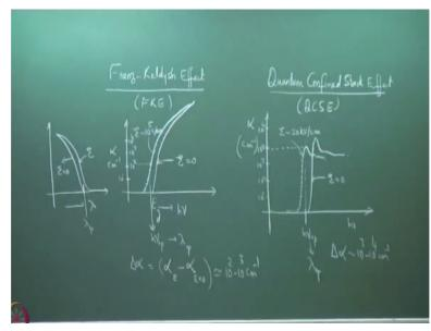
Basically, we discussed the principle of operation of an electro-absorption modulator, which is Franz–Keldysh effect and quantum confined stark effect. Both these can be used to realize electro-absorption modulators. So if you recall the characteristic of Franz–Keldysh effect is shifting of the red shift of the absorption edge of a semiconductor. If you have alpha the loss coefficient in centimeter inverse versus the photon energy h nu.
