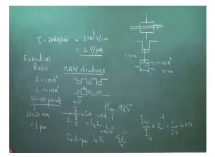
One of the early experiments at Bell Labs used multiple quantum well structures MQW structures, which means you have wells, barriers, wells, barriers. So this is the well and if they are non-interacting then the energy remains the same and all the properties remain the same so typically well width d of the order of 100 angstrom and 1 the separation so this is 1 and this is d.
