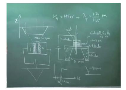
So the structure looks like this. I will show you a better, this is schematic representation. This is p side, n side and this is the intrinsic region, which comprises of quantum well structures. So the i here is MQW, the intrinsic region and then you apply a reverse bias. So pin, the intrinsic region comprises of multiple quantum well structures, typically 50 to 100 periods so if you plot the electric field across this, how does it look?
