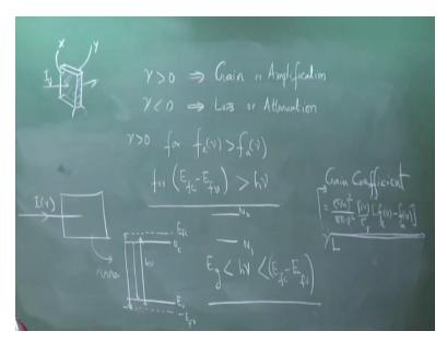
When will probability of emission be > probability of absorption? This is the condition that we have already derived and so gamma is > 0 implies gain or amplification, and gamma < 0 that is negative implies net loss or attenuation. And therefore, it is the sign of gamma which is important and which will be determine that? It will be determined by this factor fe of nu-fa of nu, and so gamma is > 0 or fe of nu > fa of nu, and this happens when?
