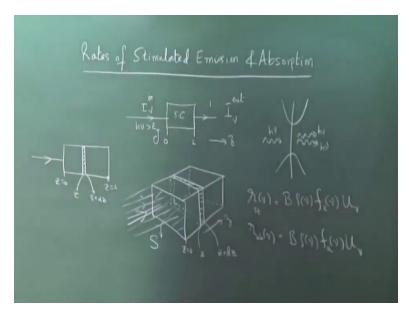
So today we will discuss the rate of stimulated emission and absorption. Our objective would be given a piece of semiconductor, a beam of irradiance I nu of frequency h nu of energy h nu>Eg, beam of h nu here a light beam of irradiance I nu entering this semiconductor here, what is the material property effect of the material property on the beam? That is the output here if I call this as 1=0 let us say this is a z direction of propagation this is 1=0 and this is L length of the semiconductor.
