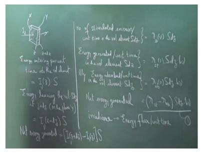
If I look at that small volume element I am now focusing on the small volume element, so let me draw the volume element here that small slice, so this is of thickness dz so z and z +dz. The number of stimulated transitions stimulated emissions let me write it stimulated emissions per unit time in the volume element Sdz= rate of stimulated emission is this one, what does this mean this tells you the number of stimulated emission per unit time per unit volume.
