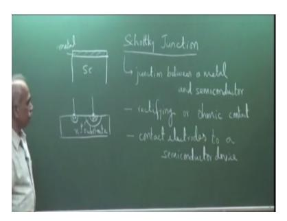
So, schottky junction refers to it refers to junction between a semi conductor and a metal, junction between a metal and semi conductor has we will see the junction could be this could be rectifying it could be a rectifying contact rectifying or Ohmic it could be a rectifying contact like a normal diode or it could be an ohmic contact we will see more on it as you can appreciate this important because it is the it provides contact electrodes or metal contact to the semi conductor.
