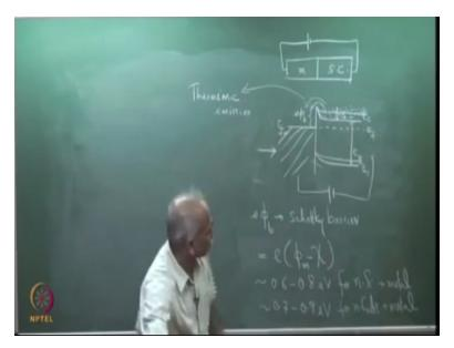
So, we apply, so the end side we are applying negative which means the energy will go up, so this band will start going up and electrons will pour over as this starts going up when I forward biase the new level is here let me show it with the slightly to distinguish let me draw after biasing the band looks like this. The upper one is after forward biasing, so what has happen the band has been lifted which means there were plenty of electrons here.
