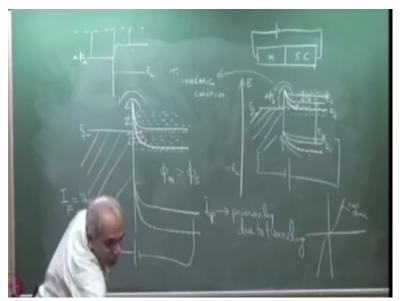
So, this is the new band diagram what I have illustrated is now you see that in this case the barrier width is very small therefore if I apply a small potential, a forward potential like this to this then of course this will get lifted and electrons can subsequently jump over the barrier but also electrons from this direction can also tunnel because the barrier width is very small. If I forward biase this will be raised and subsequently electrons can get fold into this side.
