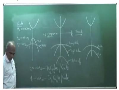
The valance band is actually more complicated it comprises of a light hole band, a heavy hole band and a split off band. So, I am now making it little bit more complicated and a split off band this is called this is the heavy hole band this is the light hole band and this is split off band the same EK diagram all the earlier was drawing I was drawing the upper most band because the electrons will get the firs field here of the holes which are interacting will be the holes which are here.
