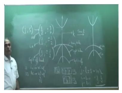
And therefore we have combination of states which are S which are J, S the states are represented by J,S which gives the combinations possible are 3/2, +-3/2 3/ 3/2 here and +-3/2, 3/2 +- half and the last one is half, +-half the first number is J, J takes values 3/2 and half S takes values +-3/2 and +-half so we the combinations which are possible are these. This is nothing but the heavy hole band this corresponds to the light hole band.
