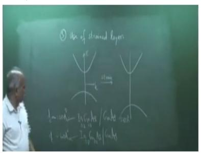
So, the third point is use of strained layers in the last class we talked about strained layer epitaxy strain layers when you introduce strain in a medium, so normally you have the EK diagram here this is the band structure in the presence of a strain what strain are we talking of at the inter phase there could be compress your strain or tensile strain, tensile strain is where it is elongated in the compressive strain it is compressed and this is done automatically.
