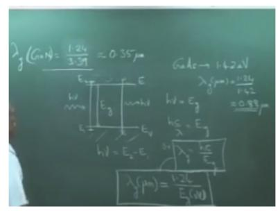
So we have Ev, Ec and this is the Eg if the photonics incidents the photon of energies hmu is is incident on the semiconductor, so this is a semiconductor which has electrons and vacant states for some electrons there, incident photon can be observed provided if I call this as energy E1 and E2 then Hmu must to equal E2-E1. If an electron sitting at energy level E1 mix an upward transition to an energy level E2.
