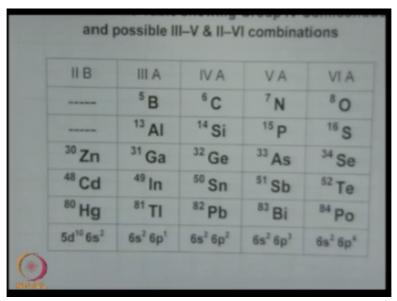
The part of the periodic table that shows group II, III, IV, V and VI elements of group 2 part of it, there are IIA, IIB and so on, but do not worry about A,B,C and so on right now group II, III, IV, V and VI. The elemental semiconductor the common elemental semiconductors combines of group IV elements.
