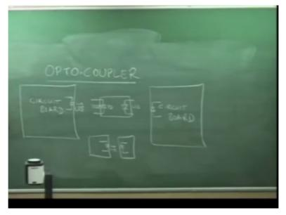
The earliest one of the earliest optoelectronic devices, one of the earliest optoelectronic devices means the optocoupler I do not know how many of you have heard about this optocoupler. Optocoupler (()) (19:55) optocoupler is a device basically is a devices at a detector here and an LED at the other end, inside small devices which is comprised of a photo detector and a light emitting diode.
