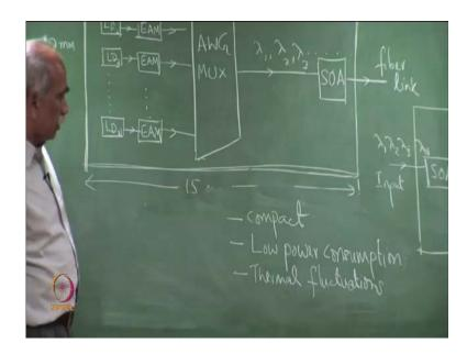
For example, the Advantages of integrating components is very well known. The first one is of course, compact it makes a compact device. Most important very low power consumption, low power consumption. Much less sensitive to thermal fluctuations thermal fluctuations, because the entire chip is maintained at unlike discreet components. The entire chip is maintained at a particular temperature and many more advantages reliability and so on.
