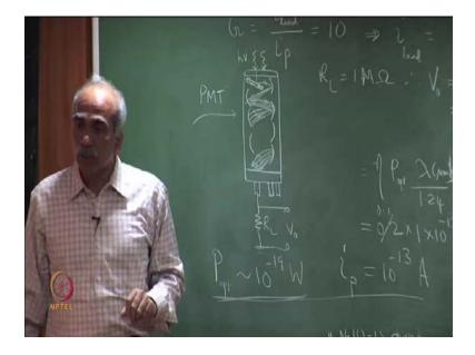
However, the current which comes out at a output, so we have a gain of 10 to the power of 7. So, gain which is equal to I at the load resistance output current divided by I primary. This is equal to 10 to the power of 7. I assume 10 to the power of 7, the number at which is calculated here and therefore, the current generated, this implies high load is equal to IP is 10 to the power of minus 13. So, this is simply 10 power minus 6 and amperes, I load is equal to 10 power minus 6 amperes.
