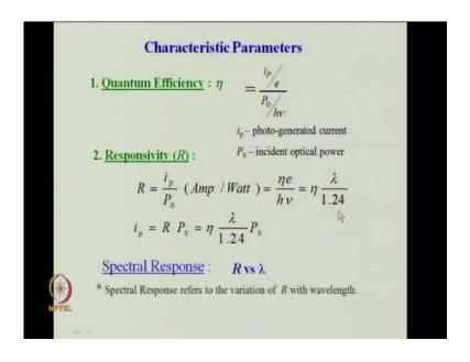
So, here are the characteristic parameters we discussed in one of the earlier classes quantum efficiency eta is i p by e by this. And therefore, responsivity R is equal to i p by P 0 which is given by eta into lambda divided by 1.24, we have already derived this. Therefore, given a material photo detector with a responsivity R, the photo current corresponding to an incident optical power P can be determined. The spectral response of
