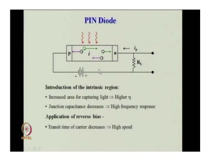
So, let us see more carefully the next slide. If we see the next slide then now, we have shown a pin diode. Why do we go for pin diode? I come back to this in a minute, let me show the diagram again. Carriers moving in side this region, inside the semiconductor carriers moving, that is electron moving in this direction, hole moving in this direction, constitutes a current in the external circuit in the external circuit.
