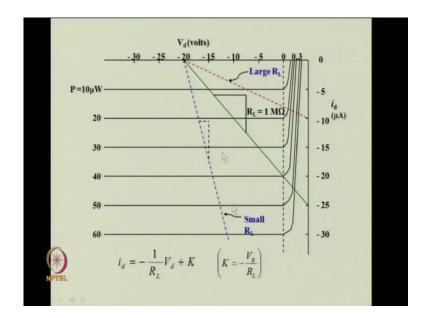
Then the next graph I have shown of plot of these, plot of the reverse characteristic for different photon flux we shown here. For a particular photo detector what is shown is only the reverse part, the forward part is here this will continue above. I have not shown I have shown only this part the reverse part, forget about the forward and what is drawn here is the load line.
