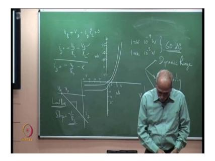
So, this is the load line how do we get the load line, if you see this here V B plus V B plus V D, V D is across the diode plus i D into R L equal to 0. So, you take to the other
