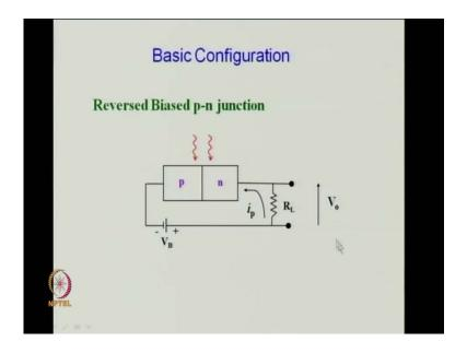
Today, we will discuss semiconductor photo-diodes and in particular we will discuss about pin-diodes. So, semiconductor photo-diodes the basic configuration is a reverse biased p-n junction, we will see why it is reversed biased, is a reverse biased p-n junction. So, as you can see there is a p-n junction here and a load resistance and this is the biased supply here and output is measured here.
