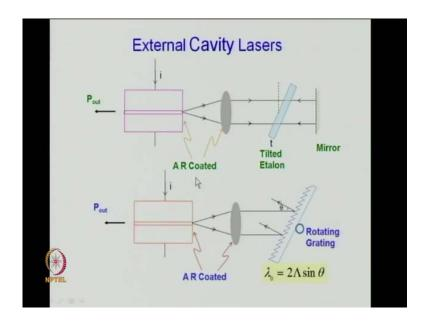
For all other wave length the light which is reflected here, those wave length which are reflected are at an angle. So, they do not go back exactly, here they may heat here, they may heat here or they may just go out. So, there is no feedback it is highly, lousy cavity for other wavelength.
