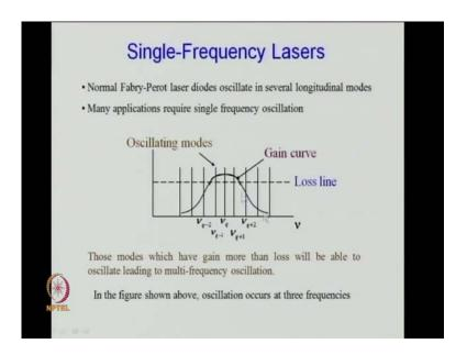
The basic idea of single frequency lasers is illustrated here; we have discussed this, but let me recall it. That normally Fabry-Perot laser diodes oscillate in several longitudinal modes, because you can see here that this is the gain curve here, and this is the loss line. And those frequencies the vertical lines represent the resonance frequencies allowed by the resonator, but only those frequencies here 1, 2, 3, these 3 frequencies have gain at those frequencies gain is more than loss.
