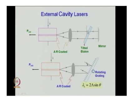
The second one which is shown here, which is shown here is a grating. So, there is no cavity here. So, this is anti-reflection coated here, if this end is the cleaved end which as 32 percent reflectivity. So, light which is going back and forth this is a rotating grating,
