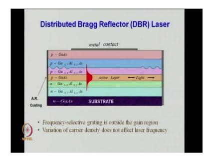
If you go to the extension that is Distributed Brag Reflector laser. This is not distributed feedback, but distributed drag reflector, what is the difference here, you can see the
