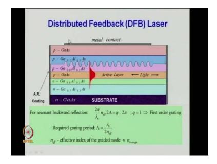
So, here is the structure which is call the distributed feedback laser, first up all it is the feedback is distributed all along the length, that is by the name distributed feedback laser. Please see the laser structure. The 2 ends are antireflection coated A R coated, the 2 ends
