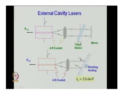
So, this is the laser here, it is A R coated anti reflection coated here, and the light output from this end passes through this. So, this is the semiconductor laser the basic device, current passes through the device and gain is provided by this medium and there is a Fabry Perot etalon Tilted Etalon, we have discussed how the tilted etalon chooses a particular required frequency. So, this is a tilted etalon in the cavity.
