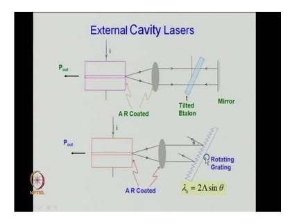
Where you will use a rotating grating here, the grating is the rotated by peso controls, by current it is not the manually rotated, it is the with the high decision you can control the feedback and therefore, the wave length which you want to choose one can use the stepper motors here to rotate this and you can choose the wave lengths in steps or you can continuously, choose the wave lengths which you want to which you want to less.
