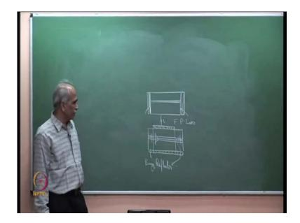
Recall the febry perot laser, the febry perot laser has reflection coming from here, from the 2 ends the febry perot. So, these are the cleaved facets, and therefore there is because it is a cleaved facet it is normally, not frequency sensitive almost all frequencies will get reflected because it is a mirror basically.
