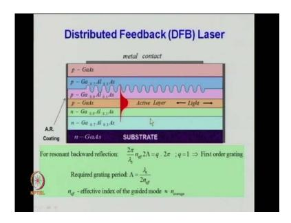
You see that the metal contact is here, carriers are flowing across, carriers are also flowing through the grating region. Carriers are flowing through the grating region which is selecting the frequency.
