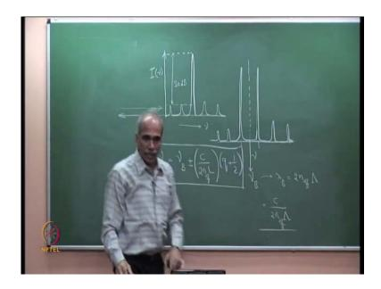
If you see the actual spectrum of a distributed feedback laser, if you see this is nu verses distributed then if this was nu b, this nu b. The brag frequency corresponding to lambda b, so lambda b. So, lambda b is equal to 2 time n effective into lambda. So, nu b is c by lambda. So, nu b here is equal to c divided by twice n effective into lambda. This is the brag wave length, but actually you see that there are 2 modes.
