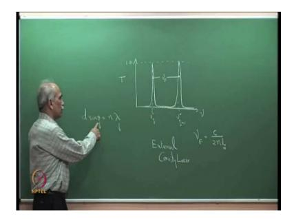
So, if you have a spectrum as you know for the grating you have d sign theta equal to n lambda. So, different lambdas will have different theta, is a reflection grating there are transmission type of gratings and reflection type of gratings. So, this is a reflection grating, in a reflection grating.
