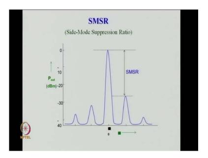
Typically, and this is characterized by a parameter we have I think I have shown here single mode, side mode separation ratio.
