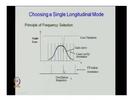
Here, you see the etalon resonance frequency are these, these are the etalon resonance frequencies separated by a free spectral range within large.
