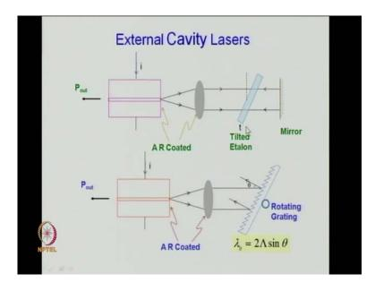
So, this is the laser cavity, from here to here this 1 is very large, and therefore the resonance frequencies permitted by this cavity are much closely placed or the free
