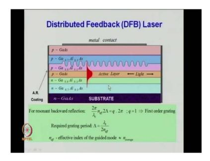
The current is passing through the grating which is selecting the frequency because the refractive index of the medium here changes due to injection current the frequency also changes with injection current in a D F B.
