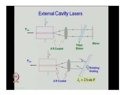
So, d is replaced by the period here, grating period 2 d 2 d sin theta equal to n lambda n is order one.
