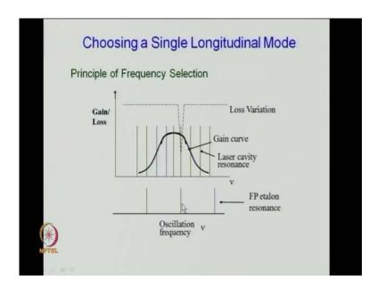
And therefore, let me go back again to the other figure here. So, these vertical lines correspond to the laser cavity and these vertical lines, correspond to the resonance frequencies of the etalon. Whenever, the etalon resonance frequency co inside with the laser cavity resonance frequency, that particular frequency will pass free real's at the cavity.
