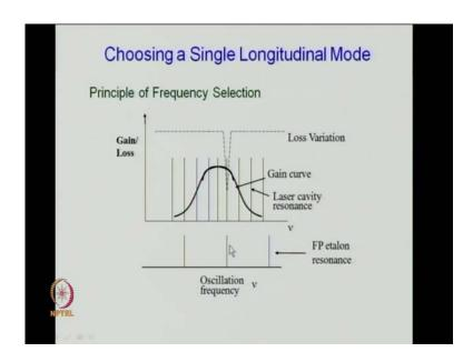
So, at least one resonance frequency this one or this one, co-insides with the laser resonance here. So, that particular frequency loss is very low, for all other frequencies here the loss is very high. So, this frequency here c is low loss because that is the transmission resonance of the etalon. So, this is the principle by, which it is the same
