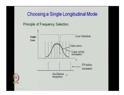
Therefore only the loss curve here, for one particular frequency. And which means here for this frequency (( )). So, gain is higher than the loss and therefore, this is the frequency which will oscillate in this place by, this means we have chosen one single longitudinal mode thus laser structure here.
