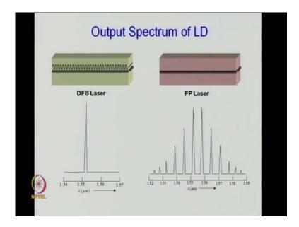
Here is the spectrum just 2 illustrate, if you take a febry perot laser is the same laser, you have the laser oscillating in multi longitudinal modes. And if you have a periodic grating here in the cladding to make it a distributed feedback laser it oscillate in a single longitudinal mode.
