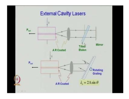
So, this etalon here, that frequency will pass through if the etalon is not there, which means for that frequency for these resonance frequencies this cavity is a low loss cavity. Whereas, for any other frequency the etalon transmission is very small, which means the does not act as a good cavity and this is the idea by which you choose, so let me go back to the figure again.
