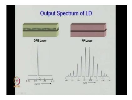
So, in a linear scale it will be just not there, that is why here I have not shown any of this, but actually there is a small amount. This is an illustration showing that it picks up one single longitudinal. So, D F B laser is a single frequency laser.
