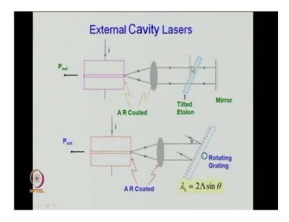
This is an external cavity laser. So, external cavity laser, which means this is the cavity, which is coupled to the laser, and therefore by using this etalon you can force the laser to
