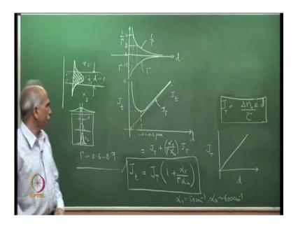
What I am now, plotting is d verses gamma. So, gamma minimum value is 0 maximum value is 1. So, for very small values of d like this, the mode is spreading gamma is closer to 0 so gamma starts from somewhere here. At 0 confinement will be 0 and it is approaching 1 as d increases gamma approaches 1. So, what I have plotted is gamma 0 to 1. How would 1 by gamma vary, when this is small this is large?
