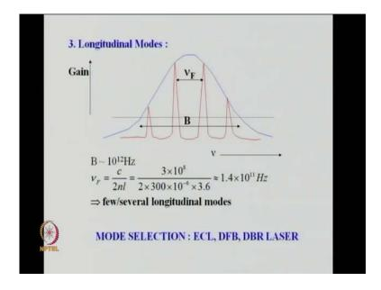
Third property is the longitudinal modes. We have had some discussion here. So, what is shown is the blue line here, what we have an shown is the gain profile the gain profile here and this is the frequency axis. So, you may recall that and this this line here, horizontal line is the loss line. So, recall what we had discuss that for all those frequencies, where so this is the loss line and then for all those frequencies for which gain gain of the amplifier.
