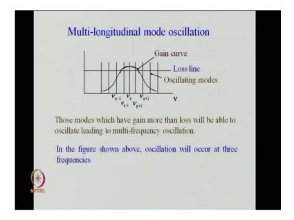
So, little bit more about towards, we are going towards selection of a single frequency. So, this we have discussed there is a gain curve. Here, the vertical lines are allowed resonance frequencies of the resonator. So, this those mode which have gain more than loss, will be able to oscillate leading to multi frequency oscillation of the lasers. So, in this frequency in this figure oscillation will occur at 3 frequencies because you can see 1 2 3. So, these frequencies gain is more than loss.
