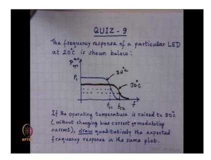
We continue with the semiconductor lasers and output characteristics. Before I start the output characteristics, let me just discuss the answer for the quiz. So, this was the quiz question. The frequency response of particular LED at 20 degree is shown below, if the operating temperature is raised to 30 degree without changing bias current or modulating current or without any change. Draw qualitatively the expected frequency response of the, on the in the same plot.
