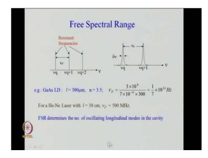
So, here is the free spectral range. Again shown clearly and typical example of gallium assonate laser diode. I is 300 micron n is 3.5. This is what we had discussed earlier. I did not know that, it was there again. For He-Ne laser, if you take He-Ne laser the common laser the l.
