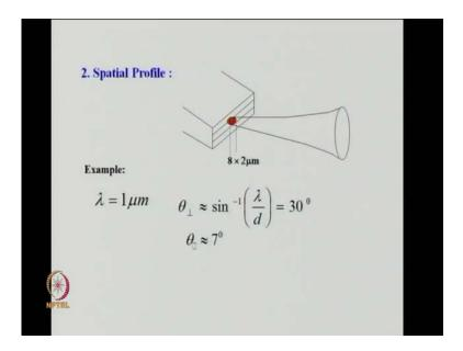
The second one is a spatial profile of the beam which is coming out, the beam that is coming out, spatial profile of the beam, right. So, the spatial profile of the beam is here. So, what I shown is the emission area here. Typical dimension is about 8 into 8 cross 2 micro meter. The spot size, this is not the physical size please remember that the double heat row structure is a just, if you see the front view we had a layer which was 0.2 micro meter here.
