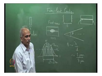
So, assume that here we have large numbers of modes oscillating like this. So, this bandwidth here is the 10 to the power of 12 to 10 to the power of 13 hertz. What about if I make that laser will oscillate in a single longitudinal mode, the width will be like this. The output, this a multi longitudinal modes and a single longitudinal mode can be
