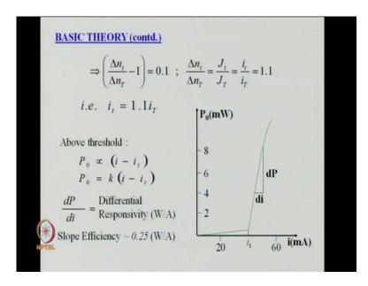
What we now bring the concept of threshold current. One is transparency current and the other is threshold current. So, both are here.
