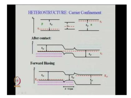
And why going to hetero structure two things which happen which you choose d therefore, 0.1 micron 0.15 micron you can choose, you are able to and because of this combination of high band gap and low band gap materials we have here, potential barriers the electron went forward bias the electron comes to this active region s, but the barrier still exist on the other side.
