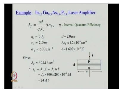
So, all the parameters are defined again here and alpha a is the absorption coefficient an example is given here this is from one of the books just taken as an example indium, gallium, arsenate phosphate laser amplifier. J T the transparency current density is e into d by eta i into tau r there was tau you recall that eta i by we had derived this expression eta i is equal to tau by tau r.
