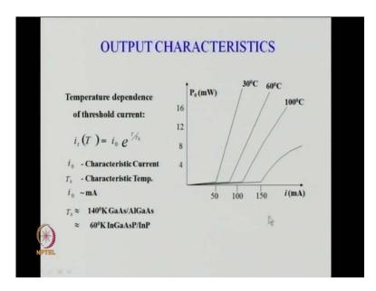
So, we come to the output characteristic earlier in the previous graph I had shown just one, but here what is shown is output characteristic with temperature and you can see that it is extremely sensitive to temperature the threshold which is here at the bottom. So, here is the threshold. So, at 30 degree if the threshold is 50 you see that at 60 degree it is increase to some 70 or 80 mile amperes. So, threshold is a strong function of temperature.
