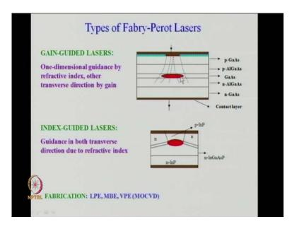
Types of Fabry - Perot lasers they are broadly classified as, gain guided lasers and index guided lasers. I have shown a typical structure of gain guided and index guided lasers. So, you can see that in a gain guided laser, as the name indicates the beam here is guided by the gain this what is shown is a front view the front view. This is the laser chip what is shown is the front view light is coming from.
