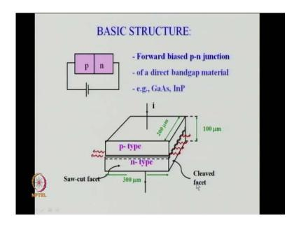
The basic structure of a semiconductor laser is as we have discussed in detail it is a forward biased p-n junction here is a forward biased p-n junction, and made of a direct band gap material such as gallium, arsenate, indium phosphate, we have discussed in enough detail, but I would like you to see the structure here what is shown with a typical dimensions. So, the structure this is the length dimension length and, this is the width dimension.
