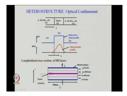
The second point, optical confinement again this is quite clear here this is this are the cladding layers which have lower refractive index this is the active region, here are the regions. So, this forms an optical wave guide which means it confines an optical guided wave which is an optical mode profile which is shown here is more profile and this is a longitudinal cross section of the laser.
