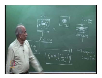
So, the structure is this. So, what is shown there is a strip which is a rectangular strip here. So, this is p this is n this is n and this is also n and in between. So, this is I and this region I should be this region because I want this region to be reverse biased. So, you have a structure which has this is n this is n and this is p this region and this region is p please see this is n p n p is the reverse biased you have applied positive here and you have applied negative here.
