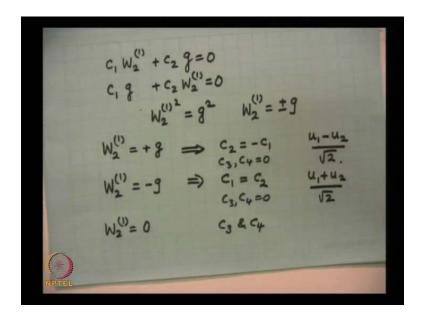
Now, first let me write down the first two equations. So, if I take the take the minus sign out, so we get c 1 W 2 1 plus c 2 g is equal to 0, c 1 g plus c 2 W 2 1 is equal to 0. So, the determinant must be zero. So, therefore W 2 1 whole square will be equal to g square and then W 2 1 is equal to plus minus g.
