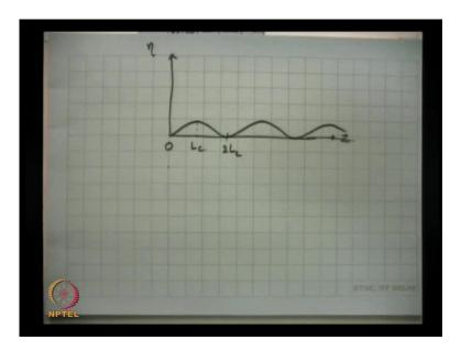
What is phase difference of pi minus 1? So, let me try to plot now. What is going to happen? If I look at efficiency versus z with delta k is equal to 0, with no Quasi-phase-matching, it was going like this; this was the coherence length.
