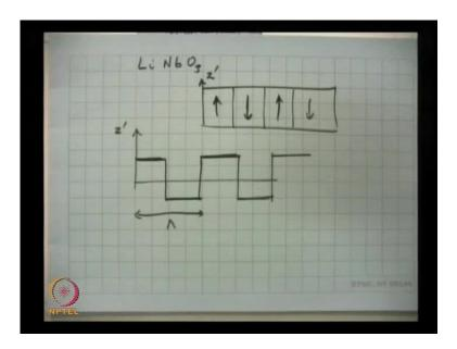
So, what I need to do is, to reverse the sign of the non-linear polarization, I need to push the lithium ion across the plane below; so, but what I can have is then, suppose, I have a crystal, I generate a crystal in which I have regions with the polarization pointing up down, up down; if I write this as my z prime axis, so, in the z prime axis, d will be positive, negative, positive, negative like this.
