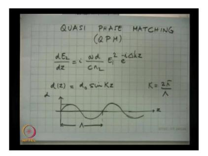
Now, remember, what was the period we had calculated coherence length? We have calculated for the lithium niobate crystal, about 3.3 microns; so, I need every 3.3 microns, the sign of d should change, so, this period is then supposed to be 6.6 microns; it is a very small period. Now, so, the first question is, of course, how do I achieve this? And, if I do not achieve exactly this, what is the result?
