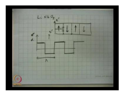
For example, I start from here; first I calculate over this distance, then I calculate over this distance; but please remember, at this point, there is both E 1 and E 2 incident; the equation which I have derived does not include this. So, I must calculate how E 1 will vary when E 2 is also present; also, E 1 remains constant.
