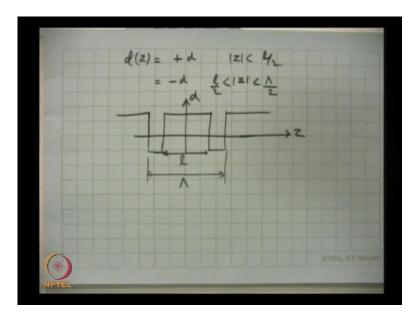
So, let me look at a d tensor like this. So, d of z, let me draw a figure here and then write the corresponding...; so, d of z is plus d for mod z less than 1 by 2, and is equal to minus d for mod z greater than 1 by 2, less than lambda by 2 (( )) yes, 1 second, 1 second; this is d z, yes, sorry.
