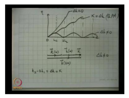
So, that I must check separately; I am assuming that d changes, and it is only that changed d that I am using in my interaction process - number 1. Number 2 is not necessary, the periods be equal, be the duty cycle be half, for example, I will show you that it is not necessary that I change every L c, I can change every 3 L c.
