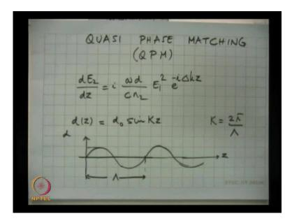
So, if I have to do Quasi-phase-matching, this must be the coherence length, because capital lambda is twice the coherence length; so, this must be the coherence length; twice the coherence length, 3 times the coherence length, 4 times the coherence length.
