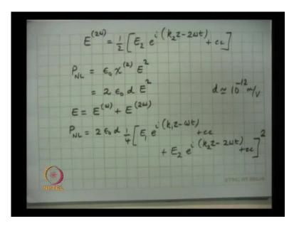
Similarly, I will write for E2, E 2 omega half of E 2 exponential i k 2 z minus 2 omega t plus complex conjugate, where E 2 is the complex electric field at frequency 2 omega; k 2 is the propagation constant of the medium at frequency 2 omega; k 1 is the propagation constant of the medium at frequency 0 mega.
