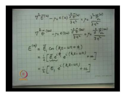
So, I will neglect the second derivative of E 2 with respect to z. Assuming that the growth of the second harmonic slow and so, this is neglected; that means, in one wavelength or a few wavelengths, E 2 does not change significantly, and that is simply neglecting the second derivative. So, I substitute this del square E omega, E 2 omega into this equation, I also calculate this second derivative with respect to time and on the right hand side here.
