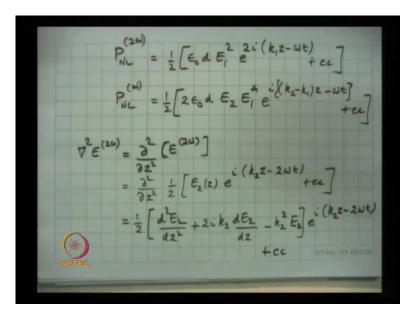
So, before we solve this equation, let me look at this term here and tell you what is the meaning of this. Where is the non-linear polarization term? Look at this equation, this equation tells me the non-linear polarization is also a travelling wave; this is also travelling wave, k z minus omega t. Now, what is the velocity of this wave?
