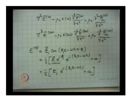
So, whether phase change is with z or amplitudes change is with z, E 1 will change with z. So, E 1 is a complex electric field; and the electric field at omega is written as half of E 1 plus E 1 exponential i k 1 z minus omega t plus its complex conjugate.
