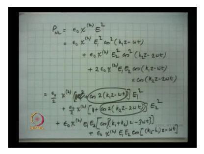
And as I will show you the phase matching condition, for omega to 2 omega conversion is the same as the phase matching condition for 2 omega to omega conversion back. That is, omega plus omega giving you 2 omega and 2 omega minus omega giving you omega, are the same phase matching conditions.
