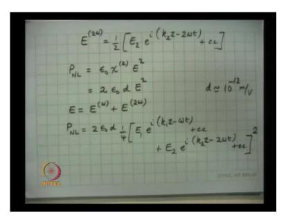
So, if I forget about the vectors, so I have expression for electric field, I have an expression for P non-linear at 2 omega, I must substitute into this equation and simplify. To get an equation for the development of E 2 as the function of z, I will get a differential equation for E 2 of z.
