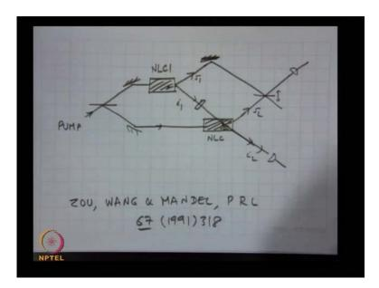
So, I have a beam splitter, this is pump lights, so then I have two mirrors here which make the beam go horizontal, here I have a non-linear crystal which generates parametric
