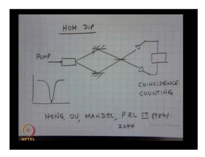
And as you move away from this position, one of them arrives earlier than the other and so within the open window of this detector one of them goes here and the other one goes here for example. So, there is a finite probability of coincidences between the two detectors but if you come into a state where both of them arrive simultaneously on the beam splitter you will either have both the photons here or both photons here and the coincidence becomes minimum.
