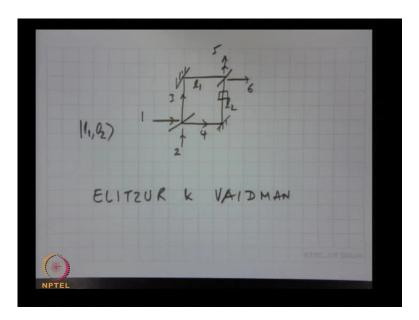
I can use this interferometer to do an experiment and give you a bomb which is 100 percent correct, good and without exploding, the idea is the following. Imagine I set up this interferometer such that as we had done if 1 2 minus 1 1 is equal to 0, if I send a single photon from here, where does it appear? Only in 6, if 1 1 is equal to 1 2 because this path and this path you can see are in phase and this path and this path will be out of phase by 5 (Refer Slide Time: 05:15).
