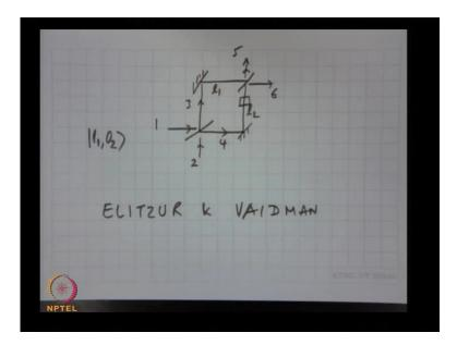
Let me recall, what we did was we had a 50 percent beam splitter generating a superposition of transmitted and reflected states then, they are reflected by 2 mirrors and then recombined another beam splitter.
