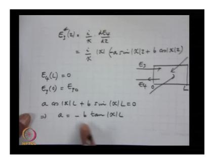
So, let me get the final solution for E 4 of z E 4 of z is equal to now a is minus b tan mod kappa 1 so, this implies a is equal to i kappa by mod kappa E 3 0 star tan mod kappa 1 i have substituted the value of b in this equation to get the value of a in terms of E 3 0 star.
