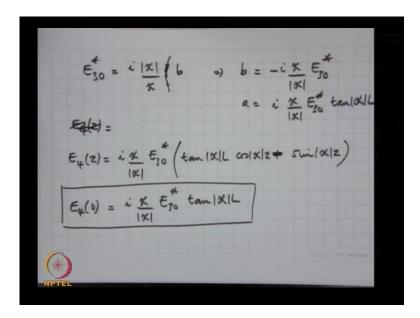
What I am interested in is what is the value of E 4 at this point because beyond this once E 4 comes out it just going to propagate backwards there is no more generation of E 4 or modification of E 4 so, what is in its E 4 of 0. E 4 of 0 is equal to i kappa by mod kappa E 3 0 star z is equal to 0 that is 0.
