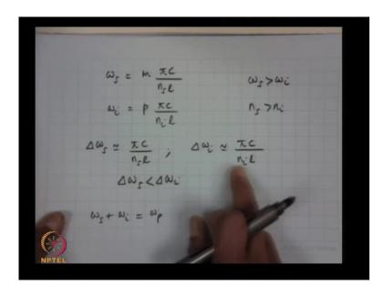
These two figures I have scaled such that omega s plus omega i at any value is omega p. Now in these figure I let me draw the lines corresponding to this omega s and this omega I remembering that this spacing's are given by these.
