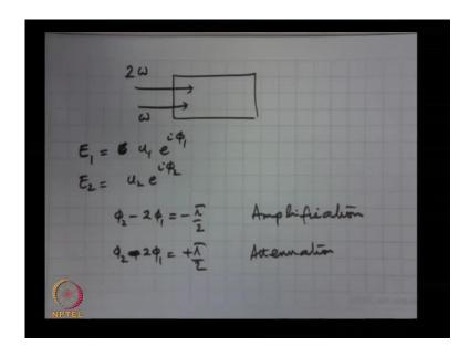
What I want to show you is, suppose I taken, let me go back to the old problem where I had a 2 omega-omega system; so, I have 2 omega coming in pump and omega. So, this is what is called as a degenerate optical parametric amplifier, because in this case omega s is equal to omega i, and omega p becomes 2 omega. The same situation as before, except that now, the signal and idler frequencies are the same.
