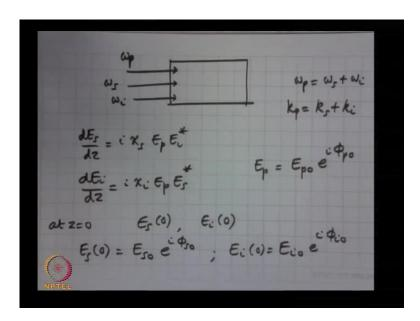
So, we will continue with discussions on the parametric amplifier. Let me recall, we are looking at a following situation, where there is this non-linear crystal, you have a pump at omega p, you have signal at omega s and idler at omega i coming in.
