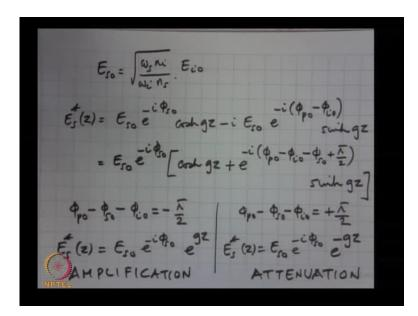
So, if I take this electric field amplitude of the idler, then I have equal numbers of signal in idler photons and trigger crystal. So, what are these imply in my solution? Look at this factor, E i0 square root of omega s n i by omega i n s. So, this actually this implies that, let me write it the other way around, this actually implies, E s0 is equal to square root of omega s n i by omega i n s into E i 0.
