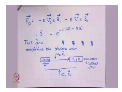
This ponder motive force is the charge of the electron into velocity of the electron due to the one wave cross magnetic field of the second wave, e m wave. And similarly, you can multiply this v due to the scattered wave and magnetic field due to the first wave. These are were the terms which that were ignored in the process of linearization when we solve the response of electrons to the to the e m wave.
