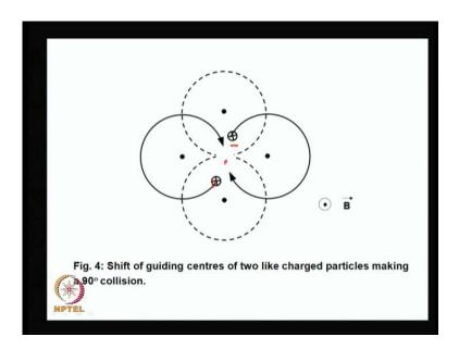
This is the figure which shows the collision of like particles, this is one particle and this is the other particle, they are gyrating, they collide and their paths shift in a manner that, the center of mass remains the same it is stationary, it is a 90 degree collision between the particles.
