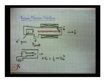
Let me just mention a something about the beam plasma system. Consider a beam plasma system, it is a very important and simple system to a study basic physics of parametric instabilities and other non-linear phenomena. This comprises primarily and electron gun here, that launches an electron beam and then, there is a chamber here which is placed in a magnetic field. So, these are the simply schematic representation of
