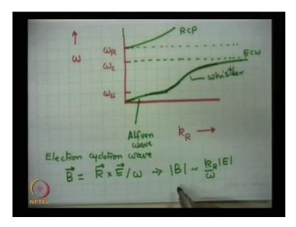
So, we have learned different characteristics of electromagnetic wave in various frequency domains. Let me plot a graph of frequency versus k. I will plot omega here and k for the right circularly polarized wave here. What I am saying that the frequency of interest r 1 is called ion cyclotron frequency omega ci which is three or orders of magnitude are more smaller than omega c. So, omega c is somewhere here. And then there is a right cut off; omega r.
