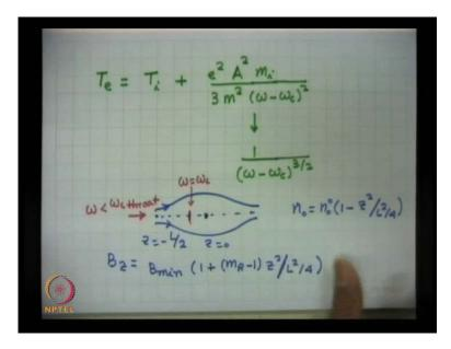
So, the heating rate one has... So, the electron temperature rise is equal to the initial temperature or ion temperature plus a quantity which turns out to be equal to e square, which turns out to be actually A square of this wave divided by something like I think 3 into 2; this becomes like I think 3 m square m i divided by omega minus omega c whole square. And this term, as I mentioned to you, because A decreases A square decreases as
