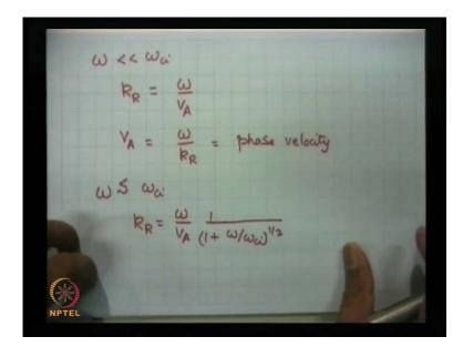
So, this is the right circularly polarized Alfven wave when it travels along the field line and so let me just explicitly write this that for omega less than omega ci, the propagation constant of the right circularly polarized wave becomes equal to omega upon v Alfven. So, v Alfven is equal to omega by k r which is called the phase velocity of the wave.
