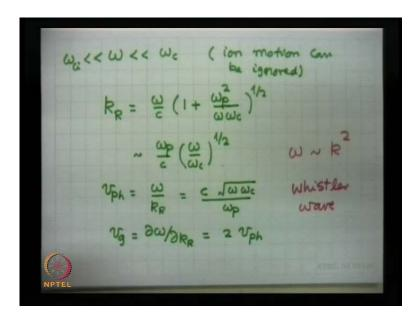
Now, let me look into the waves of lower frequencies. So far, we have ignored the ion motion. We still can ignore the ion motion if omega is omega less much less than omega c, even then you can ignore ion motion, if this is still bigger than omega c i; the ion cyclotron frequency. This is called intermediate frequency range.
