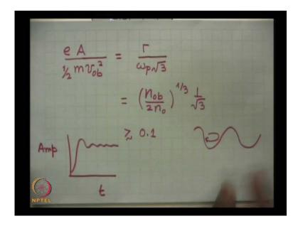
So, use this value of omega in this expression, then you can get the value of A the amplitude of the plasma wave and the result turns out to be let me write the result. It turns out to be e A upon half m v 0 b square, this is the potential energy of an electron maximum potential energy of an electron divided by the initial energy of the kinetic
