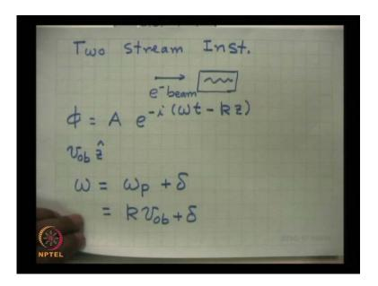
Let me begin with the remarks on two stream instability this we studied earlier for a non relativistic electron beam, we considered that, if there is a plasma through which an electron beam is launched then it gives rise to generation of waves in that plasma. The wave in the plasma we called it as a plasma wave with a potential phi we wrote down as some A exponential minus i omega t minus k z. And the beam had a initial velocity v 0 b
