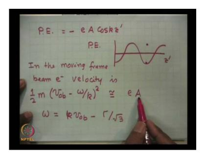
Potential energy is minus e A cos k z prime and if I plot this quantity as a function of z prime potential energy plotted here then this quantity will be like this. So, there are regions of minima and this is where the potential, which is minimum what will happen, as the wave amplitude grows with time initial then this amplitude well this potential
