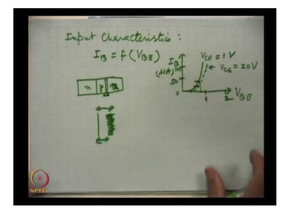
Now, first we talk of the input characteristics; input characteristics for that this is plotted these characteristics are plotted I B as a function of input voltage V E and we can plot and here this is V BE and this is I B and this is normally in Micro Amperes for example, 100, 50, 0. 0, 50 and here it is 100. This is the voltage; this is 1 volt and 2 volt. Now,
