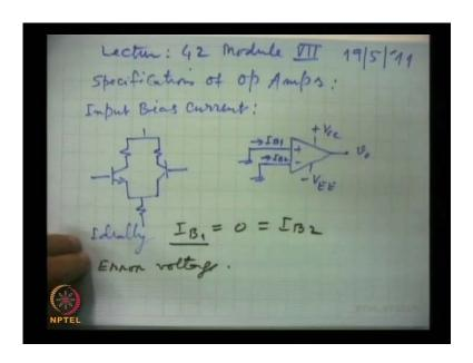
The specification of op amps, the first specification about which we talked that was actually input bias current input bias current, and this is (No audio from 01:05 to 01:17) when we do not attach any external voltage at the inputs, even then some output is observed in op amps.
