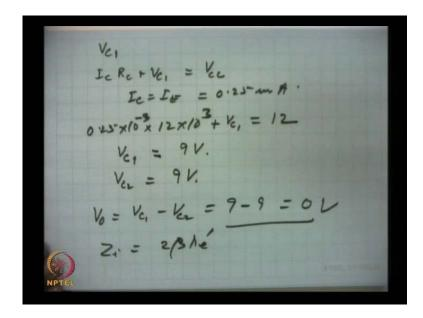
Now, to find out the potential difference between the two collectors, we apply, we find V c 1 the collector of first one is at what voltage, we apply the summation of voltages for this circuit and that gives I c R c plus V c 1 equal to V c c. I c in all B j t's I c is equal to I E, so I c equal to I E, which is equal to 0.25 mille ampere. So, this current we substitute here 0.25 into 10 to the power minus 3 in to R c, R c is 12 k, so 12 k and plus V c 1 equal to 12.
