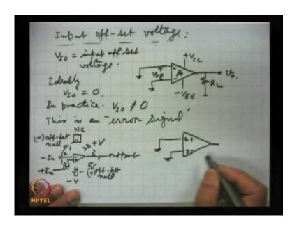
So this is input offset voltage, this is another important specification. Now, this input offset voltage is the differential input here (No audio from 07:55 to 08:22). This this input offset voltage is the differential input here, V I o offset, V I o is the input offset voltage and again this arises, because of the mismatches.
