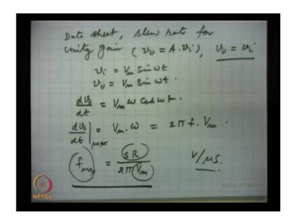
Now, manufacturers they define the data sheet the data sheet of the op amp by the manufacturer, they give slew rate for unit gain for unity gain; by unity gain is v 0 is gain in to V I and if gain is unity, then V 0 is V I; for this the data sheets give slew rates. So, let us take a sinusoidal signal v I at the input value and the peak value of v m sin omega t and same as output V m sin omega t then d v 0 d t will be V m omega cos omega t.
