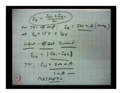
The input bias current by manufacturers is defined as the average current I B as I B 1 plus I B 2 by 2 and this is specified for various op amps. For example for 741 op amp I B is given as 500 nano amperes. This is the maximum current this is the maximum current at V c c equal to 15 volts same as also VEE when both the voltages are plus 15 and minus 15; then the maximum base input base current is 500 nano amperes.
