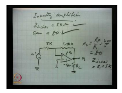
Inverting amplifier such that input impedance with feedback is 5 kilo ohms and gain is 80 it is simple, this is we have to choose these 2 values rightly, this is V out, this is R L this is V c c, this is V E E this, we choose 5 k and this we choose as 400 k and apply the signal here.
