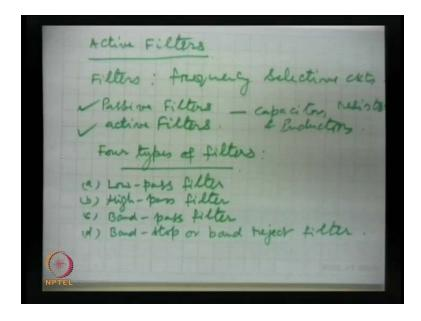
Active filters first thing is, what is a filter? Filter is a frequency selective circuit. Frequency selective; that means, you have a spectrum of frequencies and you want to select for your system that your system should respond to certain frequencies. So, how to get them? Frequency selection can be done in by using filters, filter circuits.
