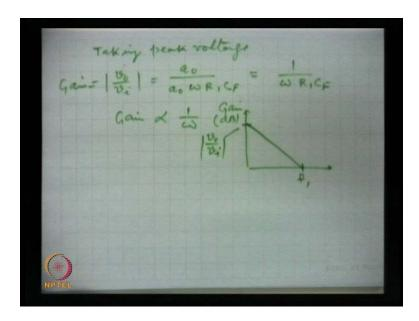
Then we can write the ratio of the two for the peak voltages, taking peak voltages both at the input and output, the ratio which is gain v 0 by v i its magnitude is, a 0 by a 0 omega R 1 C F and so, it is equal to 1 by omega R 1 C F and this is gain, gain of the intigrator.
