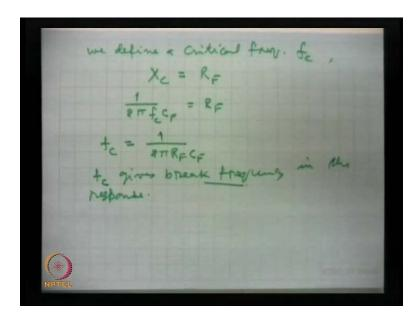
And we can define a critical frequency beyond which, integration will be alright. So, we define a critical frequency, f c we define a critical frequency f c such that, X c is equal to R F. And substituting the value of this, 1 by 2 pi f c now into C F, this is equal to R F or the frequency f c is equal to, from here 1 by 2 pi R F C F, this is the critical frequency. And this will give; f c give a break frequency gives break frequency in the response in the response.
