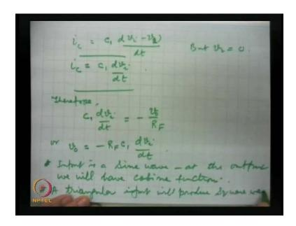
And how much is i c? The charging current charging current we can write i c, this is equal to the capacitance into, from simple capacitors theory and voltage difference, so v i minus v 0 by d t and sorry the two voltages, this is at v i and this is at v 2. So, this is 2 (Refer Slide Time: 22:10), v 2 which is 0. But, v 2 is 0 and hence i c equal to c 1 d v i d t hence, because the two currents are identical here, i c is equal to i f.
