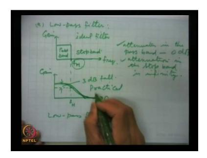
The low pass filter, first we take low pass filter. Low pass filter is the one, which is supposed to pass, by pass we mean that they will go in the circuit for further processing. So, certain frequencies from very low to a certain high frequency, they will be allowed to propagate beyond that frequency signals will attenuate heavily very heavily and they will be prohibited from going for further processing, so that will be low pass filter.
