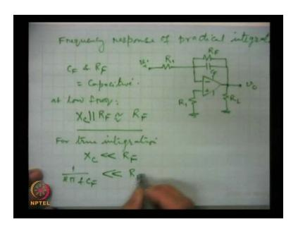
So now, we discussed the frequency response of a practical integrator, frequency response of practical integrator. So, the circuit which we are considering is now this (Refer Slide Time: 07:02), (No audio from 07:03 to 07:31) this is R F the resistance we have included; and this is C F and this is connected here and this is load across, which we take the output and here, we connect the input. So, this is the practical integrator.
