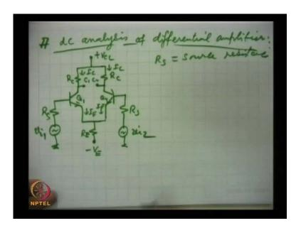
So first we take dc analysis of differential amplifier dc analysis of differential amplifier in the differential amplifier and the dc analysis the ac sources have to be grounded so the actual this is the situation this is the first source v i 1 v i 2 and this is the source
