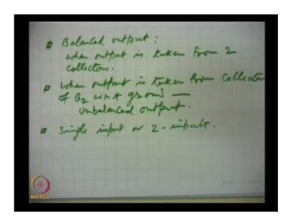
So what is balanced output balanced output that means when output is taken from two collectors this is balanced output and in fact output can be taken from one collector c 2 with respect to ground this is one possibility other possibility is when output is taken from one collector normally c 2 c 2 collector collector of this Q 2 from here we take the output from collector of Q 2 with respect to ground we call it unbalanced output.
