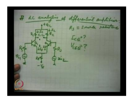
And V CEQ what are the value V CQ that is the voltage drop between this and ground here this voltage so these have to be find and for the symmetry region we are doing it only for one transistor this we have said so this is the I C now here the R s is small as I said in the beginning the source resistance is small and R s by beta will obviously be very small.
