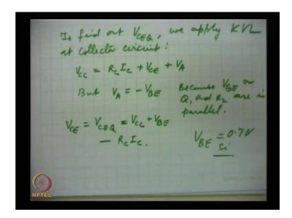
To find out V CEQ we apply kirchoff's voltage law summation of voltages at the collector circuit when we do that we get V cc V cc is equal to R C I C plus V CE plus V A where V A is the voltage at this point A what is the voltage so we have taken this but, we know this important what is the voltage here at this point A what is the voltage this is plus minus V BE this is also plus minus V BE so what is the voltage here these the voltages V BE they are in parallel.
