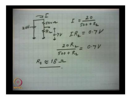
It is very simple that this circuit, We transform in this way this is 500 ohms, this is R 2 and here is that 20 volt battery 20 volts, how to find R 2 such that it produces a voltage 0.7 volts here, I am sure the problem is now clear, how to do that what is the current I
