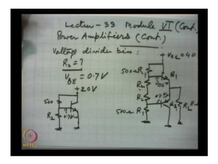
In the voltage divider wise, let us take a very simple example that how to calculate the value of that resistance. The circuit voltage divider, the circuit you will recall was this. (No audio 02:01 to 02:41) This is the voltage divider bias, let us take that this V C C is
