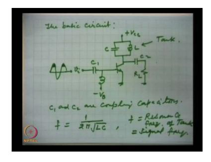
This is the circuit this is commonly used circuit for class C operation. Now here C1 and C2 are coupling capacitors the signal, input signal which for simplicity we will take sinusoidal signal.
