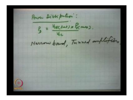
Power dissipation in that is P D this can be shown to be equal to V CE set by V CC, this is P o max, so this is also very small because this V C set is very small so but, one can calculate we have the data for these voltages and this power then power dissipation can be calculated so that finishes our class C operation and in fact this module on power amplifiers is complete, what we have is studied I am now going to summarize, we started
