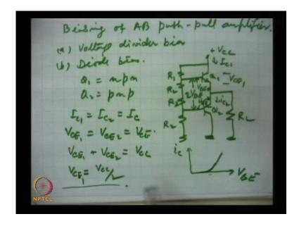
Now, briefly we take biasing of class AB push pull amplifiers biasing, there are 2 methods for biasing one is voltage divider, voltage divider bias and the other one is diode bias, now this is the complete design of class B push pull amplifier, Q1 is this is voltage
