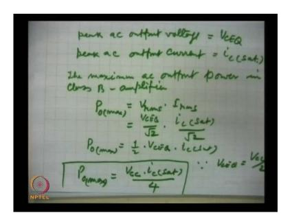
So, the peak ac output voltage is VCEQ, and peak a c output current this is ic set saturation, then the maximum ac output power will be the maximum ac output power in class B amplifier this will be Po max maximum is equal to Vrms into Irms, and voltage rms this is the peak value and hence this is VCEQ by root 2 this is ic set ic set by root 2 so this is Po maximum is equal to half VCEQ into ic set since VCEQ is V CC by 2 so Po
