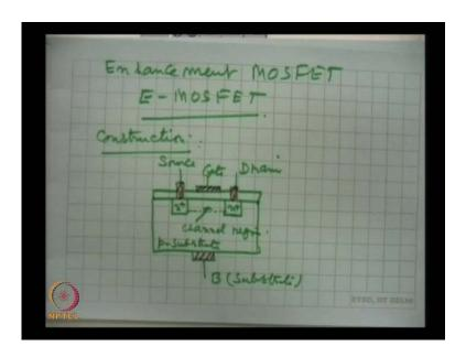
Now, we go for the next MOSFET, that is Enhancement MOSFET, which is also written as E MOSFET. First we take construction. The construction of Enhancement MOSFET is very similar to the depletion MOSFET.
