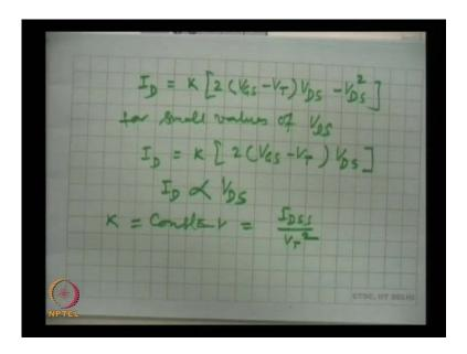
And the drain current can be shown. It is given by this expression I D, the drain current is equal to K 2 V G S minus V T V D S minus V D S square, this is the expression. And, for small values of V D S which is true for this region.
