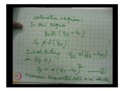
Now, the Saturation region. This is the region and in this region V D S is greater or equal to V G S minus V T. Here as the relation shows that the drain current I D is almost independent of V D S it does not depend, it depends very lightly very very little. But for the time being we may say that I D the drain current is not a function of V D S.
