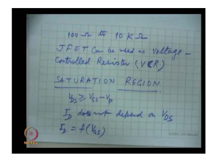
So, pinch off does not occur, but the resistance varies on the gate source voltage, the resistance in the ohmic region varies from 100 ohms to almost 10 kilo ohms. And obviously, this is a voltage controlled; it is a voltage controlled resistance, this voltage V G S, this is controlling the resistance. Here the slope is changing and which is a function of V G S and in this JFET, junction field effect transistor can be used as a voltage controlled (No Audio From: 08:20 to 08:29) resistor.
