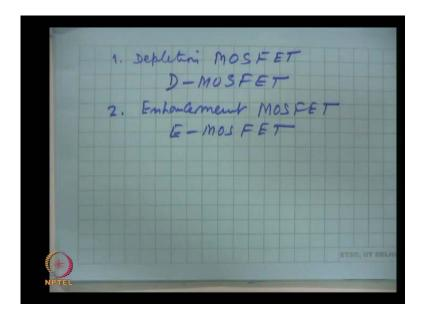
Depletion M O S F E T S, often written as D M O S F E T, D for depletion, depletion M O S F E T and second one Enhancement M O S F E T or simply E M O S F E T. There is a insulating layer which separates the gate from the semiconductor, I will give you the
