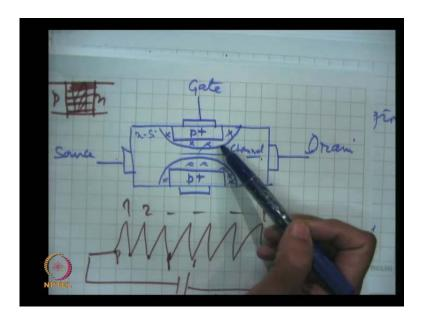
So, here the slope is changing and this you understand that when we increase the gate source voltage. This gate source voltage when we increase, this a channel conductance false, the resistance increases. For the reasons which we have discuss that, by increasing negative potential on the gate the depletion regions will a spread more, making the channel narrower.
