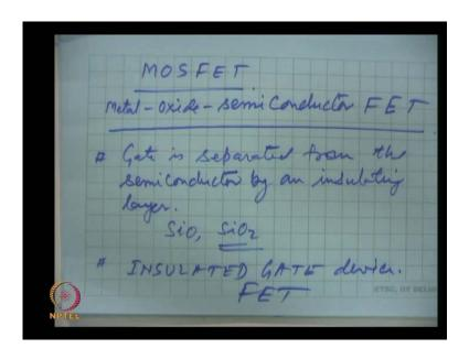
The next device in this module, which is very significant most important device today in Electronics is M O S F E T. In the beginning I have said that M O S F E T is tense for
