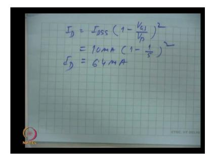
Then, the drain current again we can find out I D S S, 1 minus, V G S by V P, square. And this we can find out 10 millie amperes, 1 minus, 1 by 5, square when we solve it, it comes out to be 6.4 millie ampere, this way the problems can be handled. So, this is, about junction field effect transistor, we will return to junction field transistor again and when we talk of biasing and other things, let us talk of other devices.
