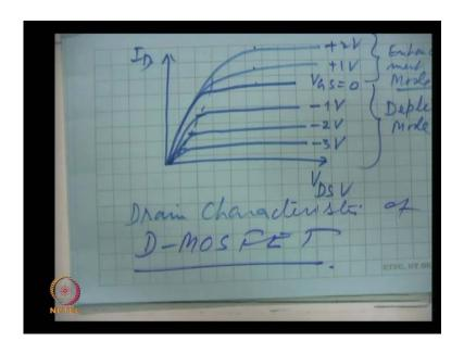
Voltage gate source, voltage is kept to 0. Then this is the channel when we change this voltage V D D, that is, V D S we change between source and drain, the current will flow because of these electrons, this is n channel, current will flow. So, this current will be this and now, this is V G S equal to 0. Now, we have given a negative voltage that reduces the conductance so, for the same voltage same drain source voltage the current will fall and this way, we will get these characteristics.
