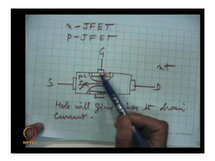
This was a F E T, this is of course P type, but it is all right. So, here now to forward bias it, we will have to give a positive potential, positive potential will forward bias the P n junction lot of current will flow so, that will not be operated. That is for n type JFET a figure must be ya.
