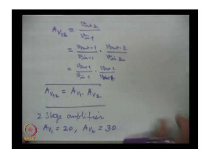
This is A V voltage gain of 1 and 2 combined that is why, i have written the gain as 1 2. And this is obviously, look at this circuit the gain the the input here is V in 1 and output is V out 2.
