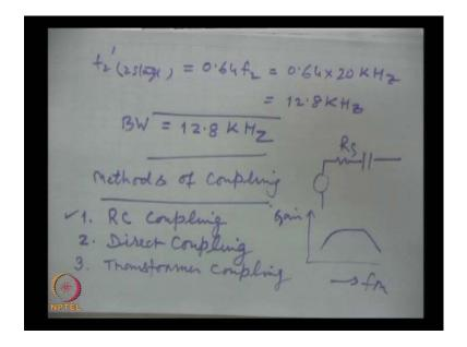
And the upper cut off f 2 prime two stage amplifier this is 0.64 f 2 from this expression 2 to the power half minus 1 when you solve it it comes 0.64. So that, this is reduced from 20 kilo hertz to 12.8 kilo hertz. And because 31 is very small so, bandwidth for this two stage amplifier actually is reduced from 20 to 12.8 kilo hertz.
