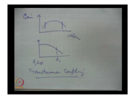
So, we talked about the R C coupling in details and a the response of a R C coupled amplifier was like this. This is gain versus frequency and these two cut off frequencies we defined. In direct coupling there is no limit on this lower cut off. And hence, the frequency response of that direct coupled amplifier is like this. Where that upper cut off of course, will be here, but lower cut off is 0 this is gain.
