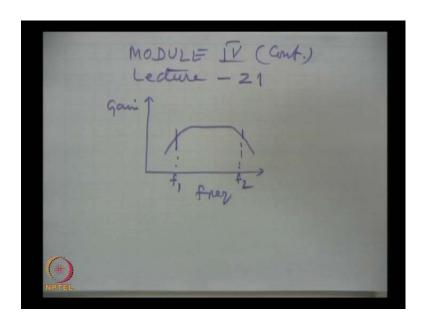
But in the graph when we plot frequency versus gain, then we get actually just one lower cut off which is f 1. Now, three factors may contribute to the lower cut off, one arises from the first coupling capacitor at the input. The other cut off may come from the second cut off at the from the second capacitor at the output. And similarly, bypass capacitor which we use with R E to enhance the gain, that may also give the third cut off. But as in the plot we get only one value f 1.
