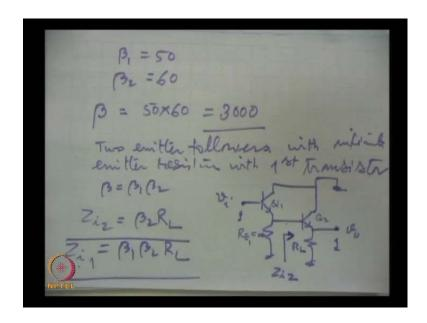
As an example, let beta 1 be 50 and beta 2 be 60, then for the compound this Darlington pair the current gain will be equal to 50 into 60, which is 3000. Darlington pair which has been formed with two transistors individually having current gain of 50 and 60. When they form a Darlington pair then, the current gain available will be 3000. This has wide applications it is formed even in integrated circuits and otherwise also in discrete circuits Darlington pair is widely used.
