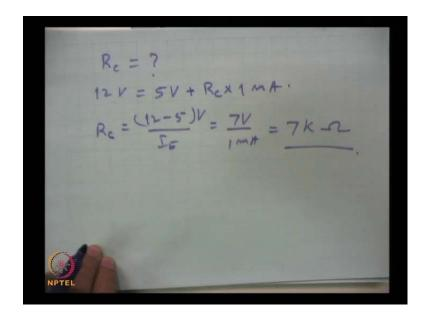
Then, R C we can find out like this, that 12 volts out of that 5 volt is the requirement that the collector should be collector should be at 5 volts. (Refer Slide Time: 42:19) And what is the drop here? I C into R C. So, plus R C into I C and I C we have found out to be 1 milli ampere and from here, we can find R C and that comes out to be twelve minus 5 volts divided by I E, which is 7 volts 1 milli ampere so, this 7 kilo ohms.
