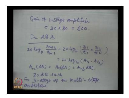
Then gain of the two stage amplifier gain of 2 stage that is multi stage amplifier. That is the product of the two so, 20 into 30 this is 600 it is the product. If we feed here 1 milli volt this will appear at the output of 600 milli volts. If the gains of individual stages are 20 and 30 so, it is a big gain.
