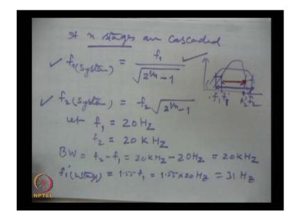
So, if n stages are cascaded, then the lower cut off for the system that means, for the multi stage amplifier this is f 1 is the cut off for the individual stage. Then this is 2 to the power 1 by n minus 1 and f 2 of the system is equal to f 2 by 2 to the power 1 by n minus 1. This is the expression for lower cut off, upper cut off of a multi stage amplifier, if they have same lower cut off(s) and higher cut off(s), if only 1 is identical then only corresponding expression is to be used.
