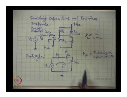
So, coupling capacitors and low frequency response (No Audio from 30:11 to 30:32). For analysis purposes only one capacitance is sufficient, actually as I said there is a capacitor at the output also that we will take little later and the circuit is this (no audio from 30:48 to 31:30). This is the C amplifier and this is the coupling capacitor, this is the source resistance which every source has and for the sake of completeness we are considering it.
