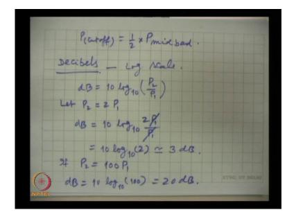
Therefore, from here we obviously see that power at cutoff P cutoff power at cutoff from here from this equation this ratio is half. So, power at cutoff is half of power at mid band that explains that these points f 1 and f 2 are half power points. So, when the power falls from mid point to half of its value then that then it cuts the this curve; it gives the lower cutoff f 1 and upper cutoff f 2 frequencies.
