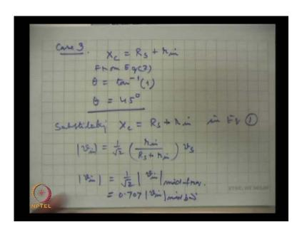
Let us examine the situation what happens when the reactance becomes equal to the series resistance of the amplifier of the circuit. The prototype circuit the R C network which we draw, this is the prototype R C network.
