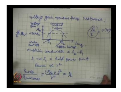
The voltage gain versus frequency response voltage gain versus frequency response for any amplifier this is a very important characteristic of the amplifier. In general we will get a response of this kind, this is frequency and this is for example, voltage gain; what does it say? We are taking that the signal frequency is varied, we start with a very low frequency and then keep on raising raising and so increase of frequency goes overs few orders of magnitude.
