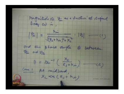
The magnitude of v in magnitude of v in as a function of signal frequency, signal frequency omega is this a magnitude of v in we take the real part of that and that is r in R S plus r in square plus X C square into v S. This is the magnitude of the signal which is going from or which is going into the amplifier. This is the magnitude and the phase
