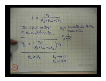
How much will be the current in the circuit, the current in the circuit is I equal to v S divided by the total resistance, because they are in series R S plus R in minus j X C; X C is the reactance - X C is reactance of the capacitor which is equal to 1 by omega C and this is when it is j then this j can be put up taking both you know you have done it long
