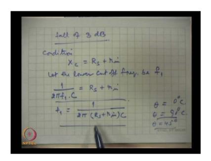
So that, this defines the cutoff this condition this condition is used X C R S plus r in or it defines the cutoff frequency. Let us call, let the lower cutoff frequency be f 1 then let us substitute for this reactance 1 by omega C and omega is 2 pi f 1 into C - the value of that coupling capacitor, this is equal to R S plus r in. From here the frequency f 1 is 1 by 2 pi R S plus r in into C.
